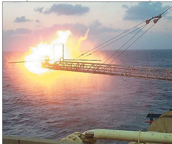
The Abu Sir-1X produced an impressive gas flare during testing sections of a 311-foot gas column. The size of the flare grew as the tests progressed and the flow rate increased. Apache engineers later calculated an absolute open flow potential at 90.4 million cubic feet per day.
