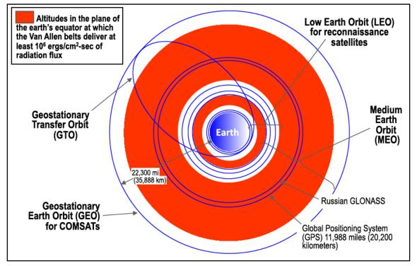
Figure 4: Earth Orbital Altitudes
