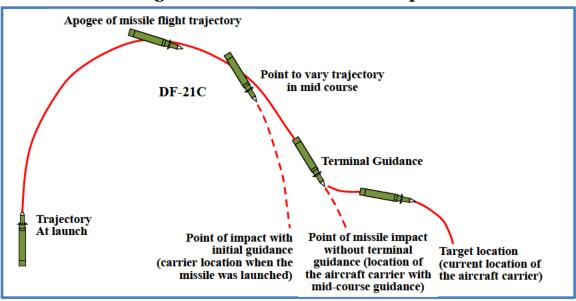
Figure 6: The PRC's ASBM Concept<sup>56</sup>
