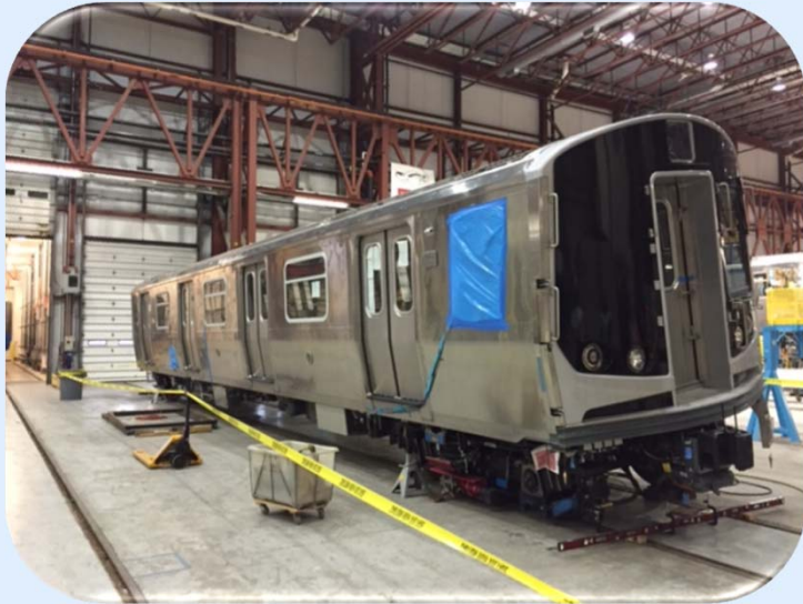
R179 car undergoing Vertical Load Jacking Tests
