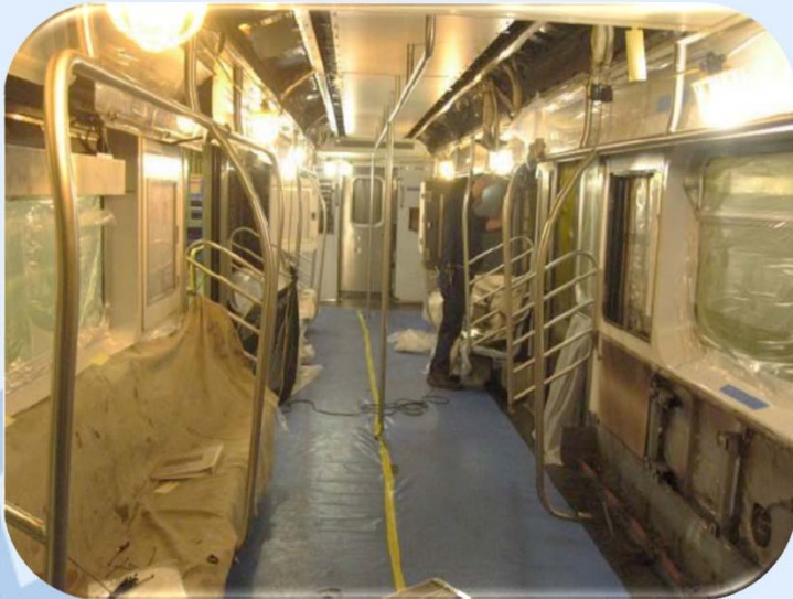
Interior Outfitting of New R188 Car
