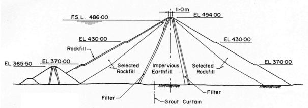
Figure 2 Dartmouth Dam Cross section
