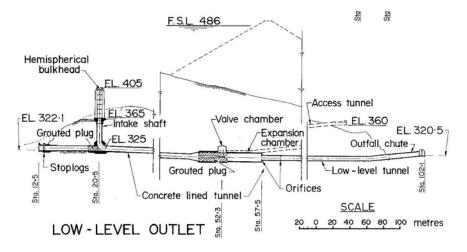
Figure 7 Dartmouth Dam Low Level Outlet
