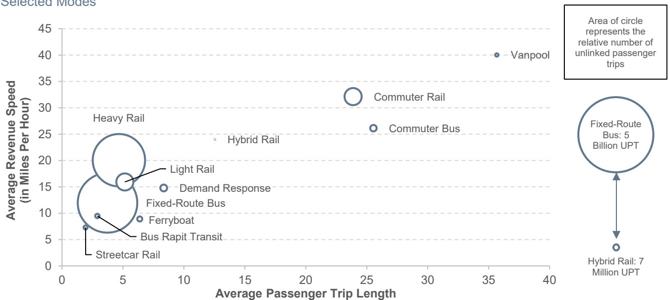
Exhibit 4-29: Transit Urban Average Unlinked Passenger Trip Length vs. Average Revenue Speed for Selected Modes
