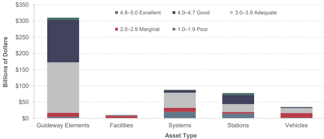
Exhibit 6-32: Distribution of Asset Physical Conditions by Asset Type for Heavy Rail
