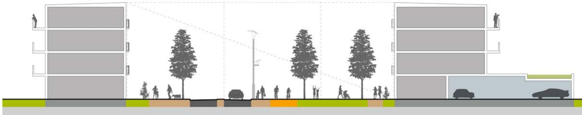
FIGURE 4.11 TYPICAL SECTION OF THE BEAM PARKWAY (AT A WIDTH OF 34M), ILLUSTRATING THE HEIGHT TO WIDTH RATIO, THE ENCLOSURE TO THE STREET, AND HOW APARTMENT BUILDINGS CAN HELP TO MAXIMISE THE AVAILABLE SPACE FOR LANDSCAPING AND THE PUBLIC REALM
