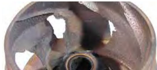
Erosion corrosion of cast iron impeller
