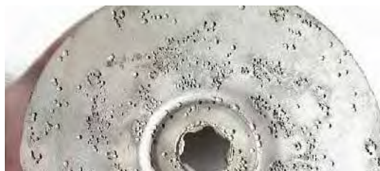
Pitting corrosion of EN 1.4401 (AISI 316)
