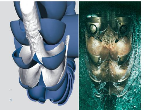
1 Simulated flow through Pelton runner 2 Actual flow through model
