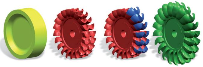
Step 1: forged disc machined
