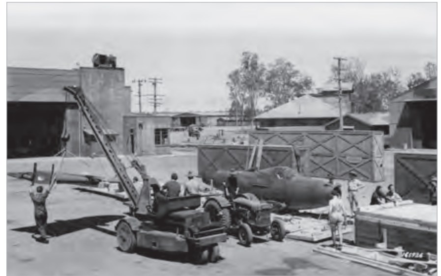
A Bell P-39 Airacobra is being removed from a crate prior to assembly. Hangar 76 visible in background to the left and the Station Headquarters to the right. (US National Archives. Image no 111-SC-165929).
