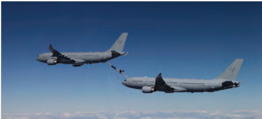
May 2015 and the first air re-fuelling boom contact made by an RAAF crew of the KC-30A Multi-Role Tanker Transport (MRTT) aircraft. (Australian Government Department of Defence).
