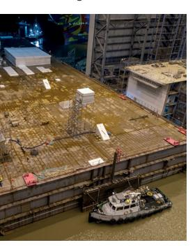
This year a total of three floating engine room units (FERUs) have already left NEPTUN WERFT for delivery to Papenburg or Turku. The FERUs are the heart of our cruise ships, containing the main machines, piping systems, refrigeration and air-conditioning systems, generating units and other components. They also include the LNG system and three LNG tanks, which comprise one of the latest and most advanced propulsion systems for cruise ships.
