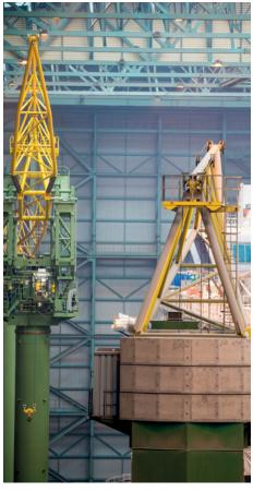
A new 16 tonne crane called "Mangokautz" has been operating in hall 6 since the start of the year. The new crane has an adjustable jib, giving it roughly 10 metres more lift than our other arm cranes. This is important in view of the fact that components are getting higher and higher. Therefore in hall 6, crane operations are now possible up to deck 20 and 60 cm below the roof.
