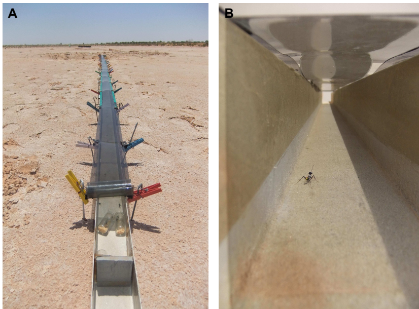
Fig. 4.2.: A Foto of the experimental setup B Close-up of the channel, the ant walks under an overhead stripe of polarized light produced by the POL filter and simultaneously sees the sun.
