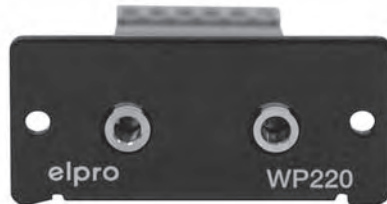
■ WP220 - Dual 3.5 mm jack vs. 3+3 poles terminal block
