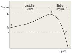
Under no load, the motor rotates at a speed close to synchronous speed. As the load increases, the motor's speed drops to a level (P) where a balance is achieved between load and motor torque (T<sub>P</sub>). If the load is further increased and reaches point M, the motor can generate no greater torque and stops at point R.
