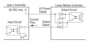
The linear motion controllers (**EZSII**, **SPV**, **EZCII**, **EZA** and **PWAII** Series) adopt an I/O specification that allows the controller to be used with either the NPN or PNP specification by changing the wiring.
