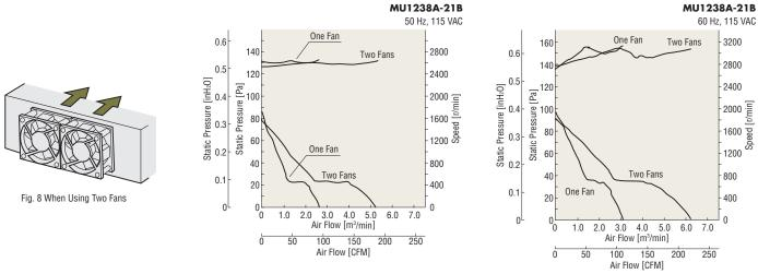
Fig. 9 Changes in Air Flow – Static Pressure Characteristics Using Two Fans
