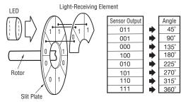
Capable of detecting absolute position within one rotation of the servo motor, the absolute encoder outputs the absolute position of the rotation angle.
