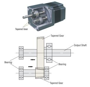
Structure of **TH** Gear's Final Stage
