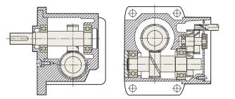
Structure of the Screw Gear in the Right-Angle Gearhead
