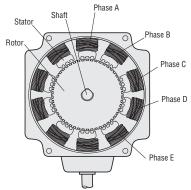
Motor Structural Diagram: Cross-Section Perpendicular to Shaft
