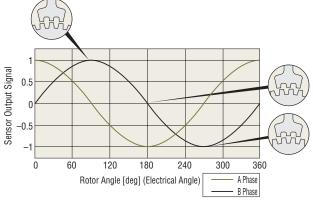
Output Signal of Rotor Position Detection Sensor
