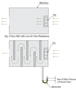
Fig. 5 Flow Path with High Air Flow Resistance
