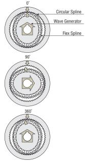
Combines three basic parts. The flex spline is bent into an oval shape by the wave generator. The teeth at the long axis of the oval mesh with the circular spline, while the teeth at the short axis of the oval are completely separate from it.
