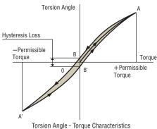
This displacement occurs when an external force is applied when the gear is stopped, or when the gear is driven under a frictional load. The slope can be approximated with the spring constant in the following three classes, depending on the size of the torque, and can be inferred through calculation.
