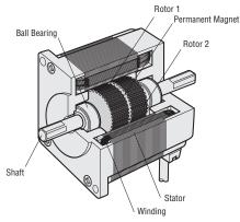
Motor Structural Diagram: Cross-Section Parallel to Shaft
