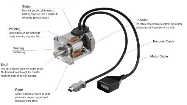
The encoder is a sensor for detecting the speed and position of the motor.
