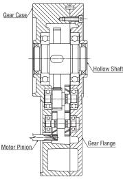
Structure of the Hollow Shaft Flat Gearhead
