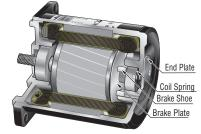
The brake mechanism is constructed as shown in the figure above. The coil spring applies constant pressure to allow the brake shoe to slide toward the brake plate.
