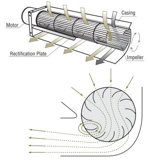
Fig. 3 Structure and Air Flow Mechanism of Cross Flow Fans
