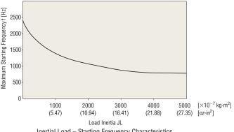
Inertial Load - Starting Frequency Characteristics
