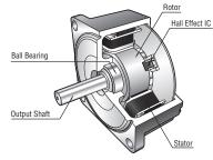
The brushless motor has a built-in magnetic element or optical encoder for the detection of rotor position. The position sensors send signals to the drive circuit. The brushless motor uses threephase windings in a "star" connection. A permanent magnet is used in the rotor.
