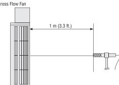
Fig. 12 How to Measure Noise
