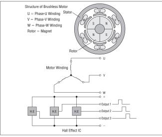
A Hall effect IC is used for the sensor's magnetic element. Three Hall Effect ICs are placed within the stator and send digital signals as the motor rotates.
