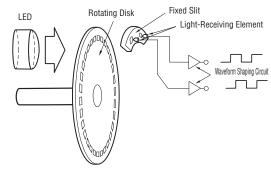
Capable of detecting the rotation, speed and rotation direction of the servo motor, the incremental encoder outputs the pulse with respect to the change portion of the rotation angle.
