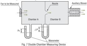
Oriental Motor's double chamber equipment is a measuring device with the highest level of general utility that may be used regardless of
