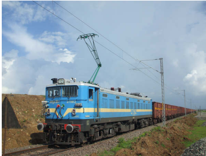
Fig. 2 : Loaded electric train running under 7.45 m OHE during test trials
