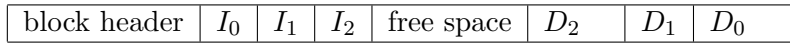
Figure 7: A leaf node with three items. The items are fixed size, but the data elements are variable sized.
