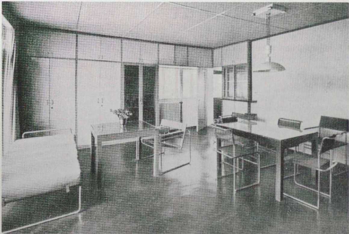
Fig. 60. Dining room, Mart Stam house, Weissenhof housing exhibition, Stuttgart, 1927. In the Stam house Breuer made use of modular enameled metal cabinets of his own design. His interiors at this time relied increasingly on metal furniture, glass-topped wooden tables, and linoleum floors.
