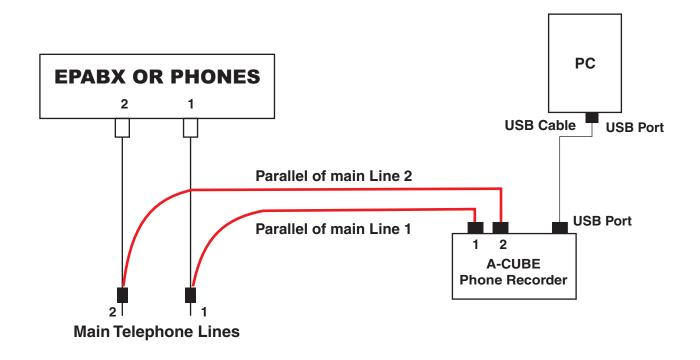
Each Parallel Cable should have RJ - 11/Telephone Connector at Recorder end.
