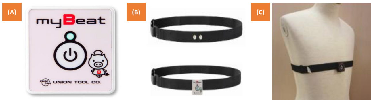
Figure 3. Wearable heart rate sensor from Union Tool Co. (A), electrode sensor connected to a chest strap (B), and position of the strap on the body (C).
