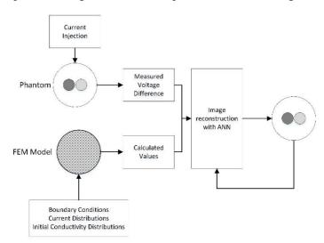
Figure 1. Block diagram for the image reconstruction process in EIT
