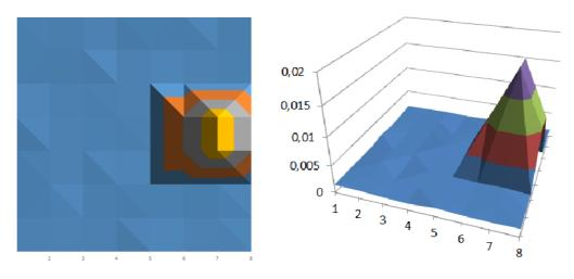
Figure 5. a) Two dimensional reconstructed conductivity image, error % 0,03 b) Two dimensional reconstructed conductivity image, error % 0,3
