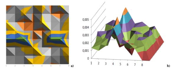
Figure 4. a) Two-dimensional reconstructed conductivity image of two objects, error % 0,05 b) Three dimensional reconstructed conductivity image of two objects, error % 0,05
