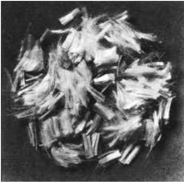
Figure 3.4 Photograph of Kevlar® Staple.
