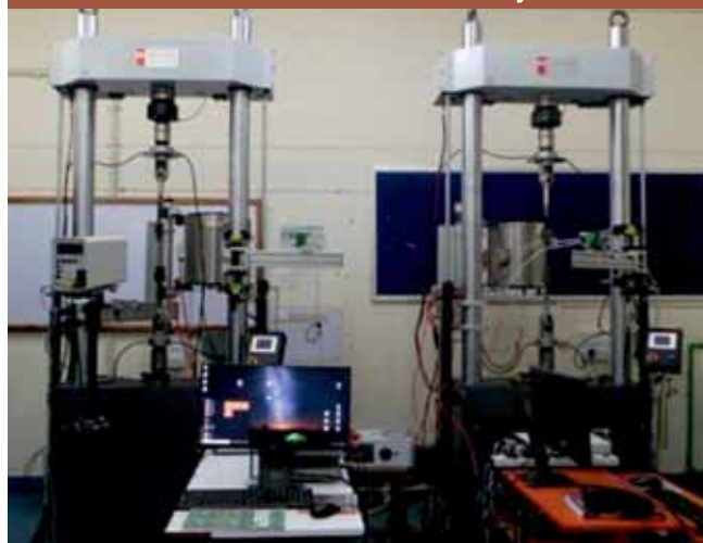
100kN capacity servo-hydraulic FCG test system
