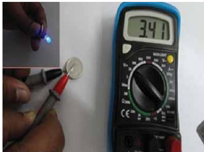
Fabricated coin cell showing the OCV of 3.4V
