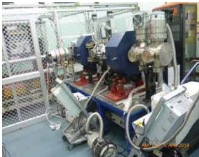
The experimental setup of Ion source coupled with LEBT
