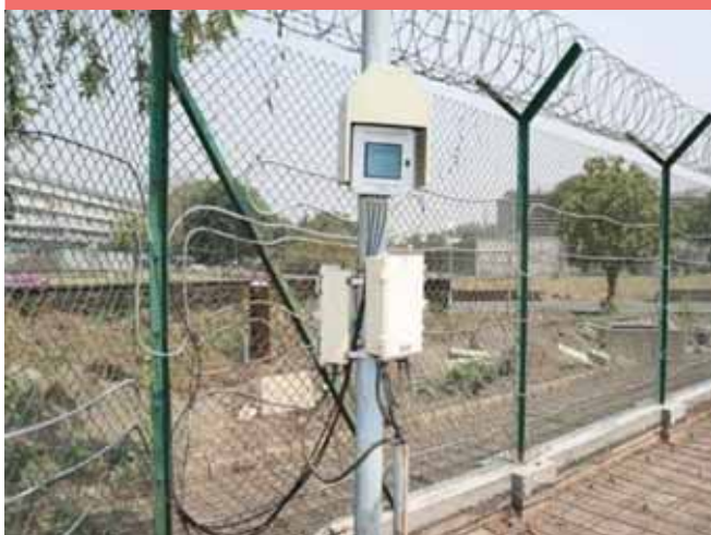
The prototype RF seeker deployed in BARC covering around 200 meter fence
