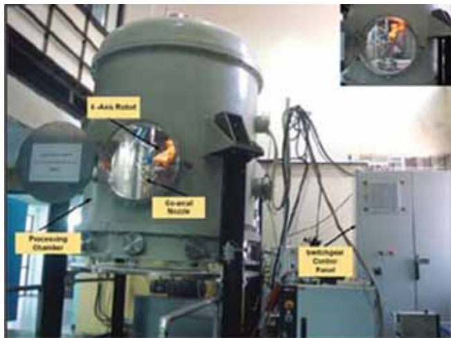
In-process large volume-laser additive manufacturing system.
