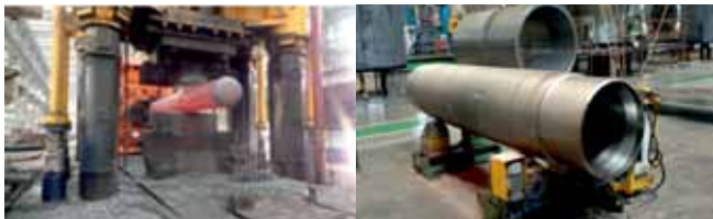
Steam Line Venturi under Forging and Steam Line Venturi
