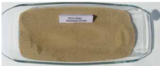
99% pure hafnium oxide (HfO 2 ) produced in BARC
