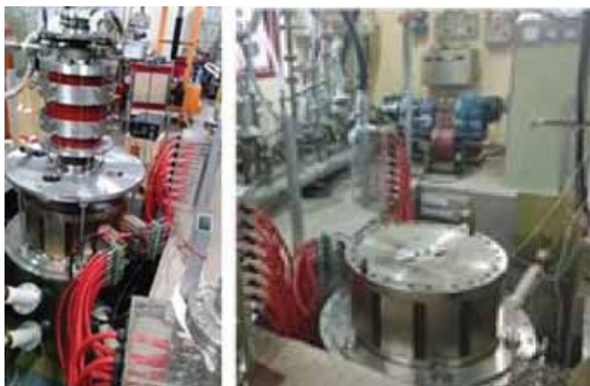
Magnet Assembly integrated with Gyrotron tube at Institute of Plasma Research
