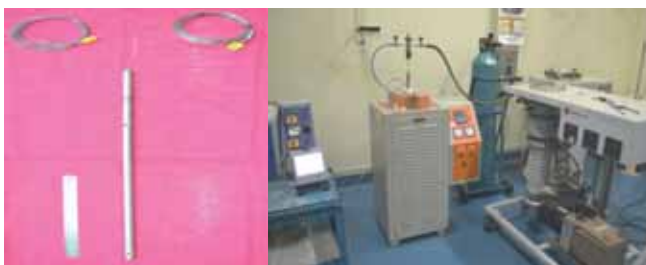
Out-of-pile version of fuel instrumented capsule (left) Testing in Electrical Furnace (right)
