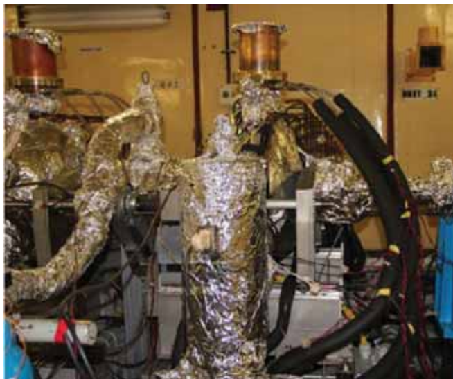
The sixth RF cavity along with vacuum system during baking
