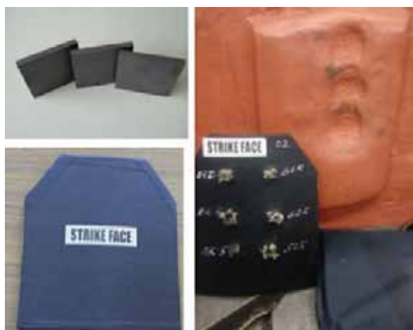
Ballistic Evaluation of B4C-CNT Composite Armour
