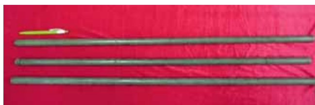
Ni-Ti-Fe Shape Memory Alloy rods of \text{Ø } 20\text{mm}
