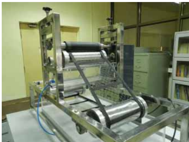
Prototype device developed for demonstration of oil-water separation
