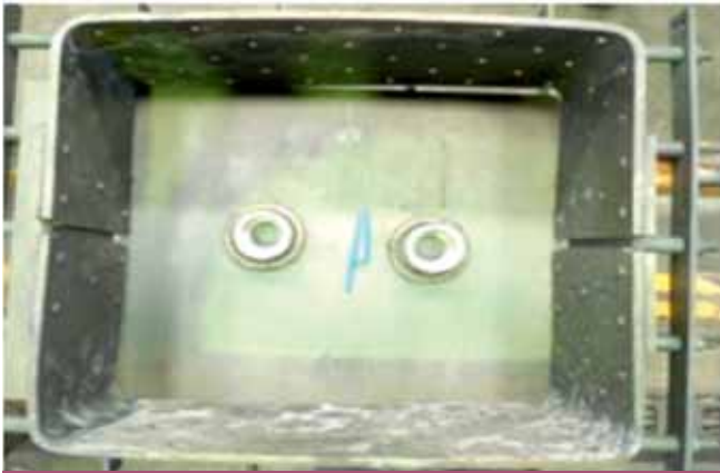
Fixture containing SmCo 5 powder compacts rings for sintering
