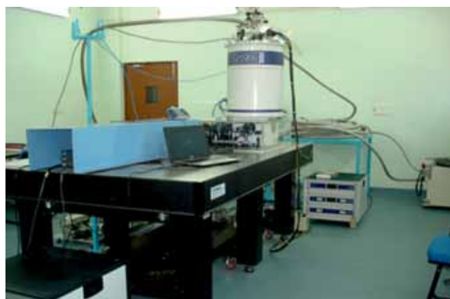
Experimental set-up for terahertz time domain spectroscopy at low temperatures and in high magnetic fields
