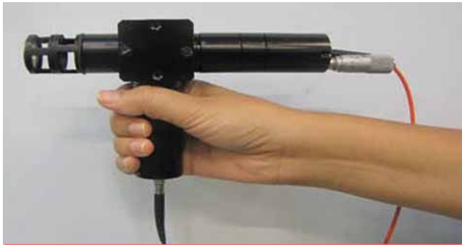
Hand-held probe for measuring depth-sensitive fluorescence signatures in a layered turbid sample
