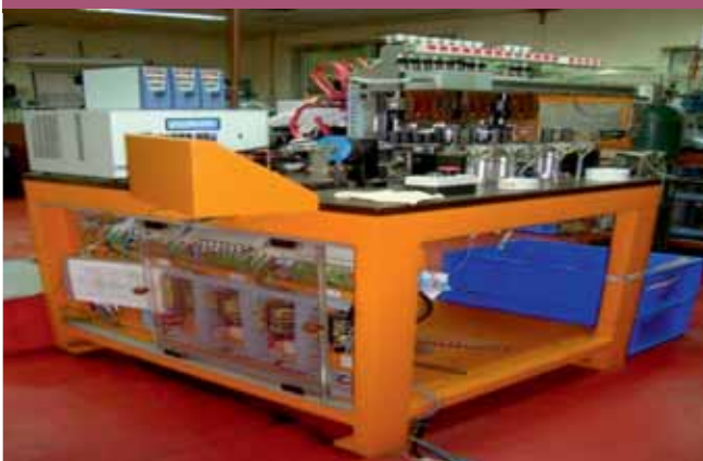
Converted appendage welding machine
