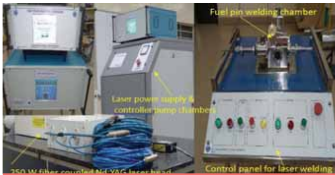
250 W average power Nd:YAG laser system for welding of fuel pins at IFF, BARC
