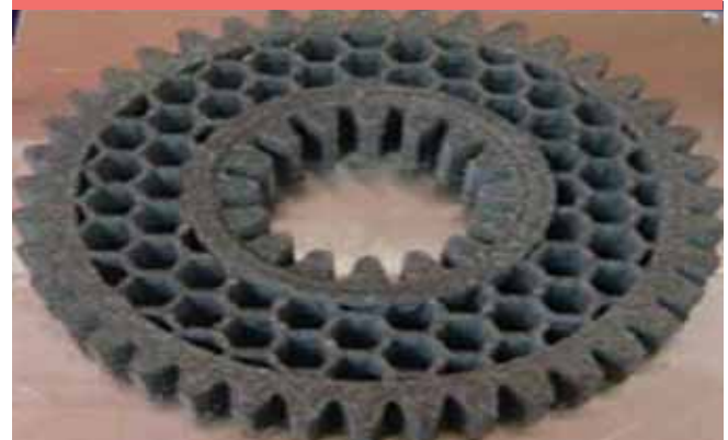
External and internal geared geometry with honeycomb core.
