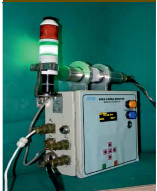
Area Gamma Monitor with CsI/SiPM
