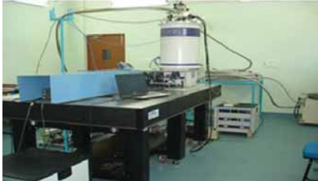
Experimental set-up for terahertz time domain spectroscopy at low temperatures and in high magnetic fields
