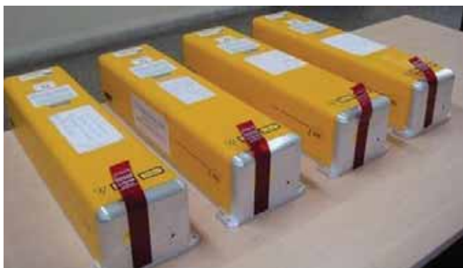
Refurbished sealed off CO 2 lasers
