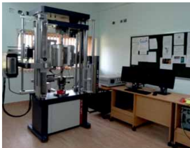
100 kN capacity screw driven tensile testing Machine with 3-directional laser-video extensometry
