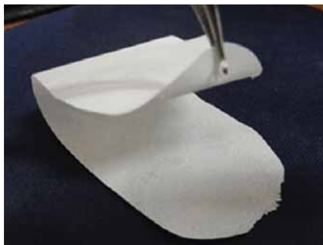
Flexible thin self-sustained polymer electrolyte fabricated using LAGP
