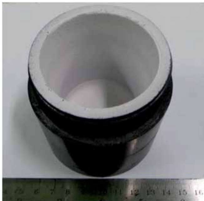
Yttria coated Graphite crucibles used in pyro-chemical reprocessing
