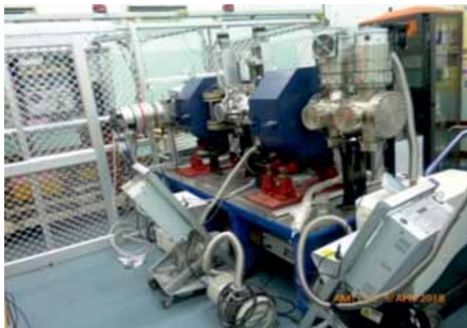
The experimental setup of ion source coupled with LEBT
