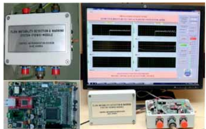
Flow Instability Detection and Warning System (FIDWS) to detect the onset of the flow oscillations in coolant channels of nuclear reactors
