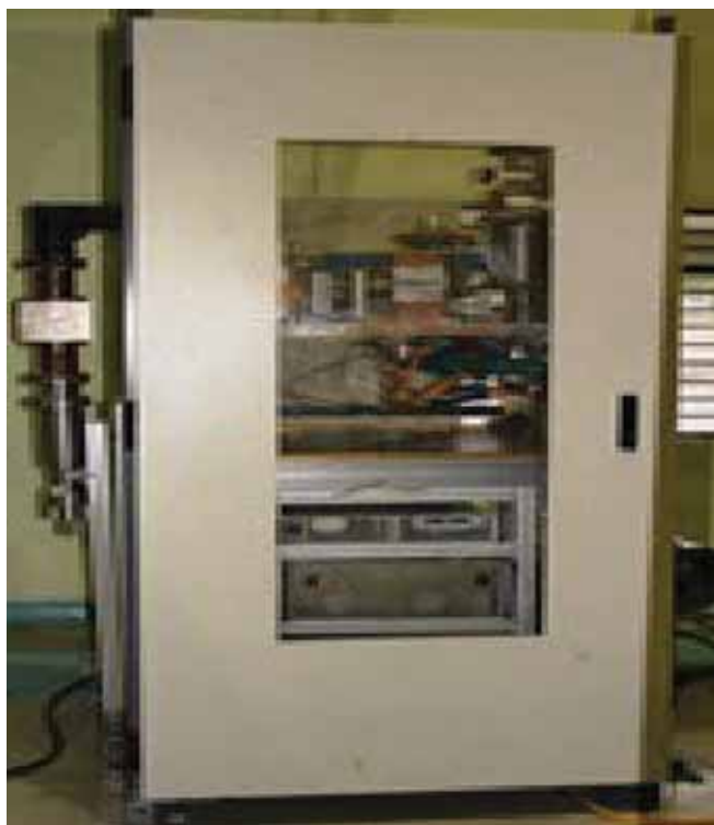
100 kW, 1 MHz RF amplifier
