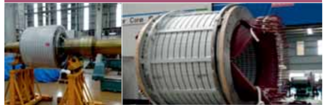
PCP Rotor Assembly & Stator Assembly
