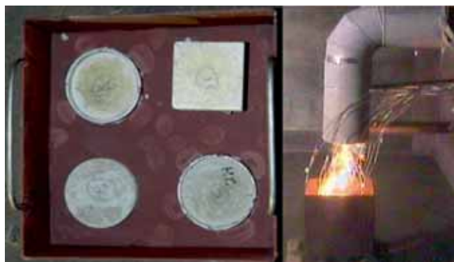
GPC Concrete Specimens; Testing in sodium fire
