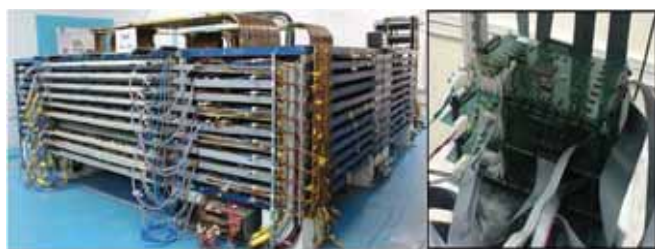
The 85 Ton mini-ICAL 1 Tesla magnet in Madurai, Tamil Nadu, equipped with field measurement systems, coil cooling systems and populated with Resistive Plate Chamber (RPC) type detectors.
