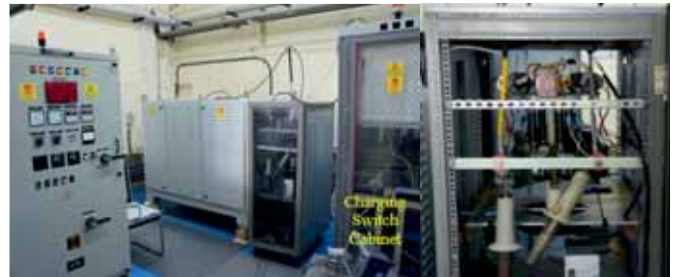
Charging switch test setup at 10 MeV Linac microwave system (left), along with the close up view of charging switch (right)
