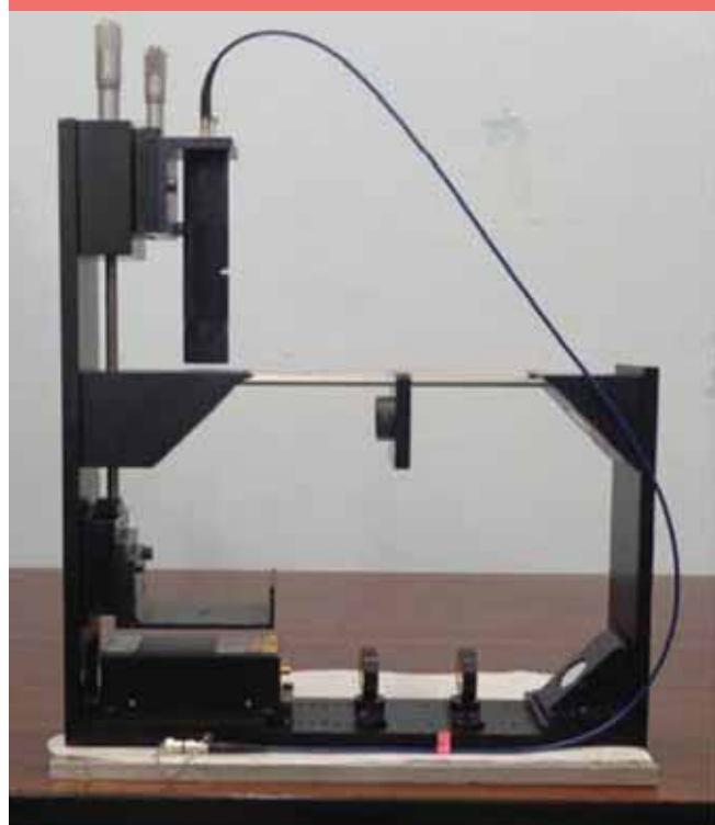
Opto-mechanical module for the measurement of Raman spectra from concealed food /biological samples
