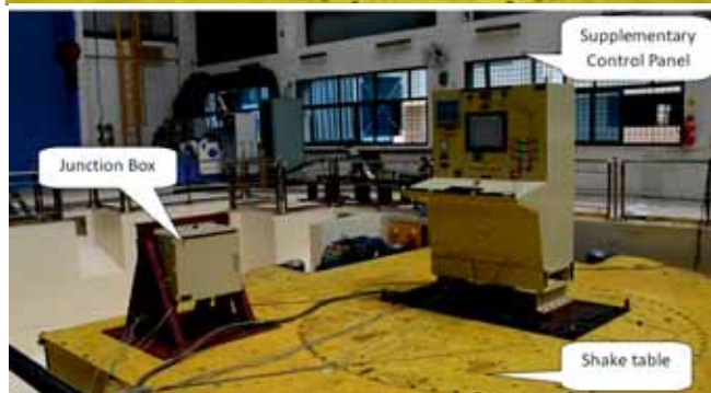
Seismic qualification tests on Passive Catalytic Re-combiner Device (Type-B1) housing along with catalytic bearing plate (above) and Seismic qualification tests on supplementary control panel along with junction box for FBTR (below)
