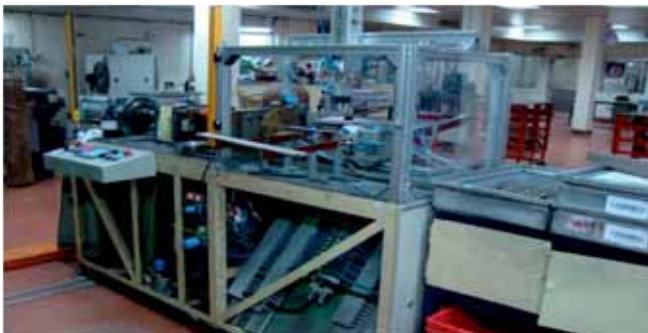
Converted end cap welding machine
