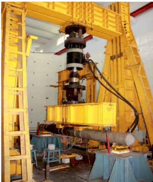
Test set up of full scale dissimilar metal pipe
