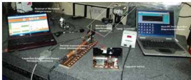
In-house developed capacitive position sensor and lab calibration setup
