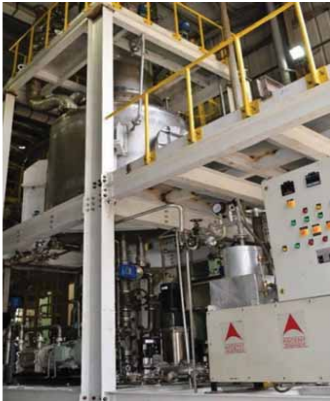
5 cubic meter/day Brine Concentrator Unit with Thermo Vapour Compressor
