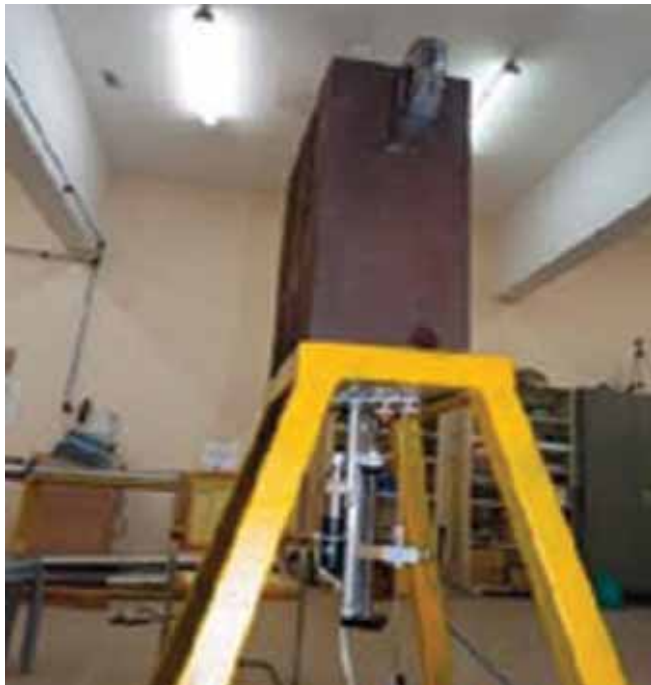
Laser cutting tool inserted in SG tube for axial grooving
