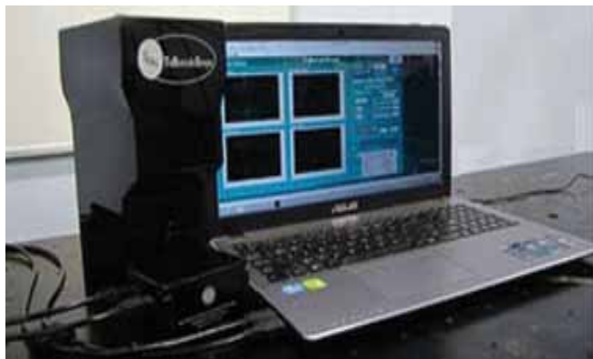
"TuBerculoScope" along with the graphic user interface on a laptop
