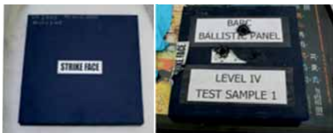
Ballistic Shield before and after ballistic test
