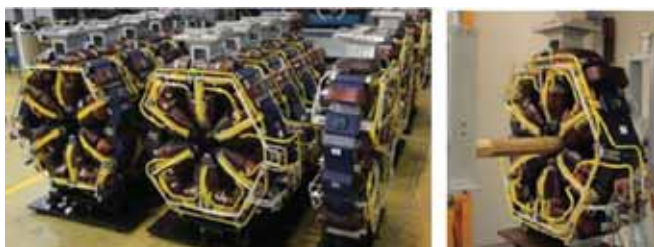
Harmonic sextupole magnets, showing coils of sextupole, skew quadrupole, horizontal and vertical fields (left) Magnet characterization on rotating coil harmonic bench (right)
