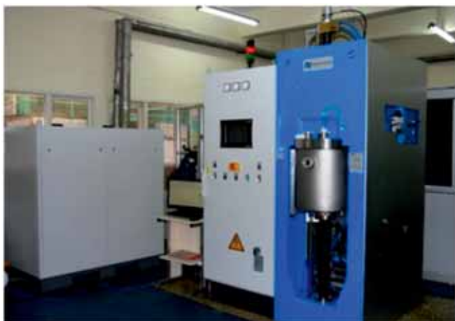
Spark Plasma Sintering Facility at IGCAR used for WC pellet fabrication
