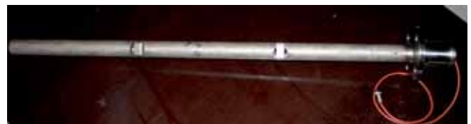
A level probe of range 0 to 1000 mm
