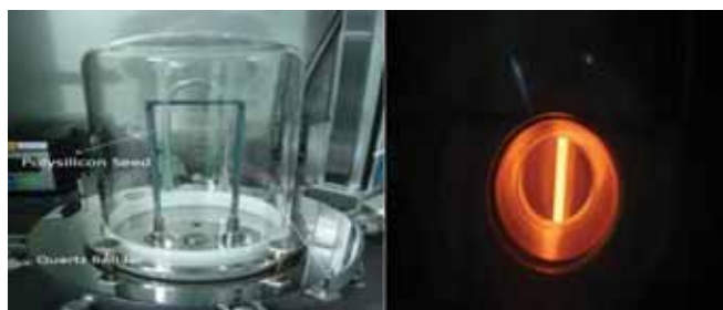
Quartz bell jar reaction for chemical vapour deposition of high purity silicon rods
