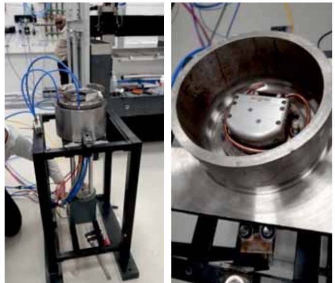
Single Pass Laser Welding Setup with Rotating Laser Welding Head (LWH) inside the Prototype Assembly
