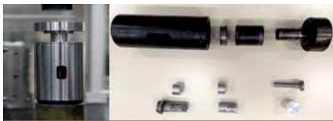
Miniature hot extrusion setup mounted on 10-ton compression testing machine (left) Expanded view of miniature extrusion setup and extruded forms (right)
