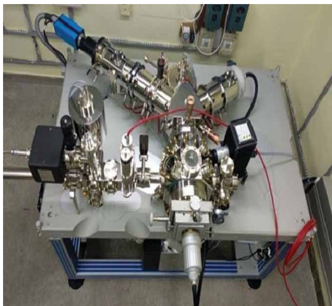
Commissioning of the Low-energy Electron Microscope cum Photo-Emission Electron Microscope (LEEM-PEEM) facility at SINP
