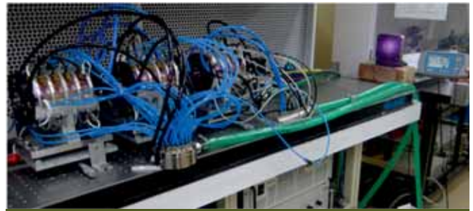
High power (2.5 kW), multi-module Nd:YAG Laser
