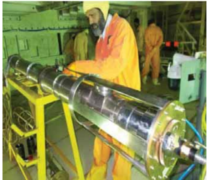
Laser cutting tool for bellow lip mounted on coolant channel
