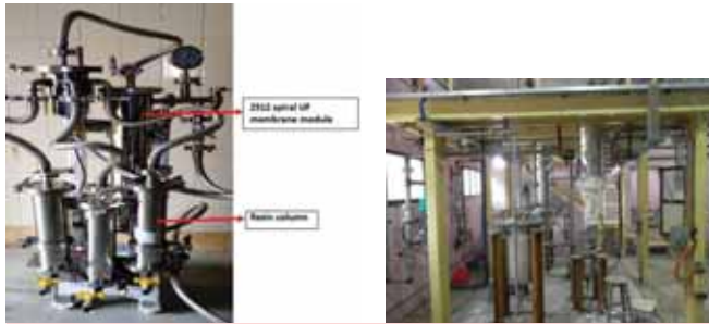
Ultrafiltration (UF) Membrane manufacturing set up in AFFF, Tarapur
