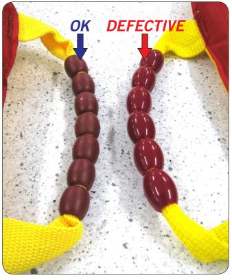
Defective Beads can be visually identified by their shiny appearance and quantity of 6 on the PFD handle. PFDs with 7 matte beads on the handle are not affected.
