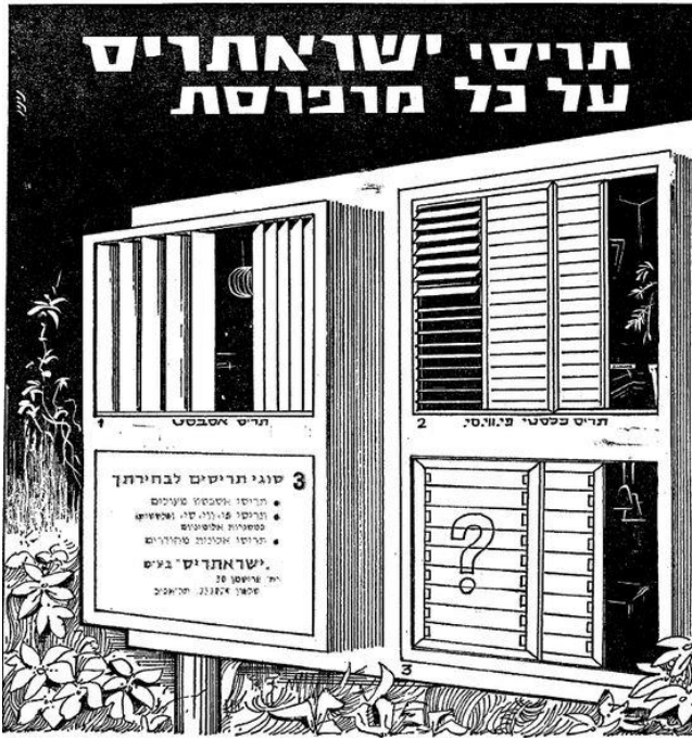
Figure 4.28: A newspaper ad illustrating the product range of the shading devices company Isratris, marketing side by side asbestos cement and PVC-aluminium shutters ( Davar Supplement for the Levant Fair, 24.6.1964, p. 19 )
