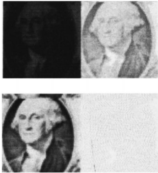
Fig. 18 Experimental sensor outputs with dual sampling with four row delay yielding exposure ratio of 15:1 for two different levels of faceplate illumination. The left images are the output of short integration channel, and the right images are the output of long integration channel. The upper pair has lower faceplate illumination than the lower pair. Note vertical shift between the left and right images corresponding to a four-row delay.
