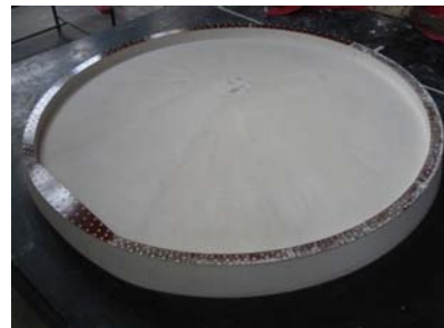
Fig.6. Assembled view of master model before tool layup
