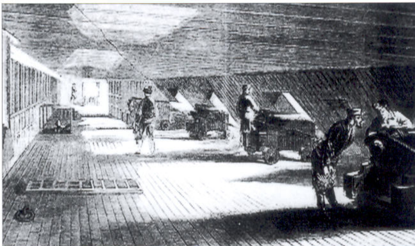
A view of the gundeck of the City Class vessel USS Carondolet , looking aft. The cabins shown on the left ran along the centerline of the ship, and would be dismantled before a battle. (Author's Collection)
