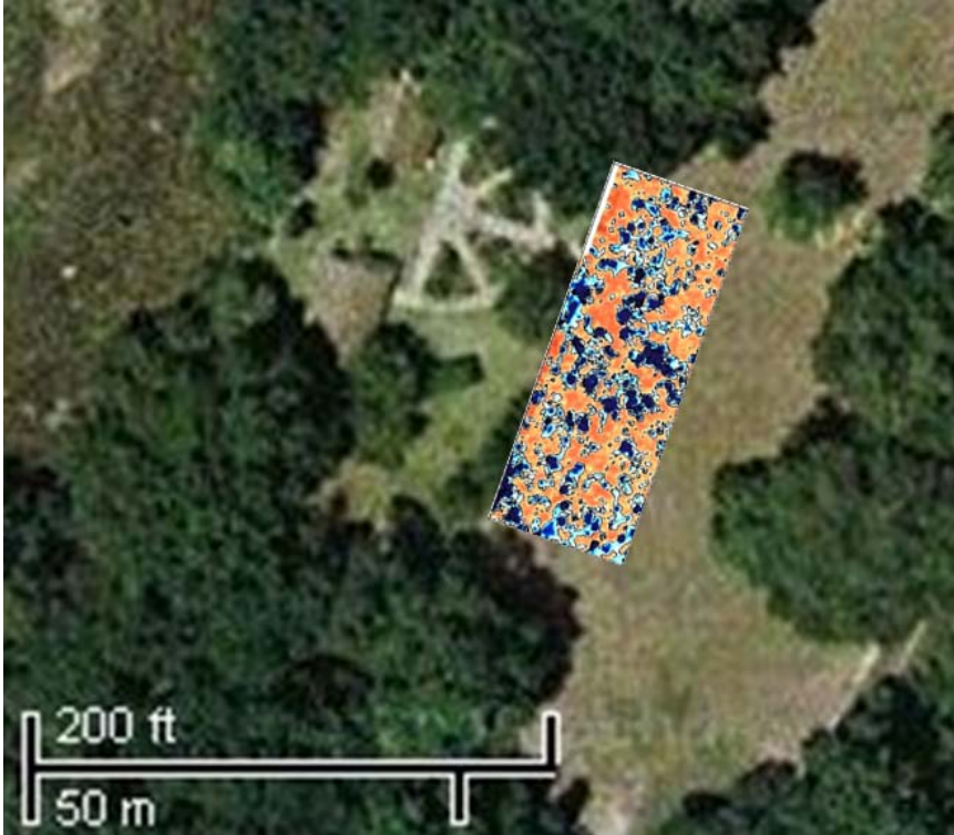
Figure 9. GPR Overlay Map (27-31 ns) on Aerial Image of Gascoigne Bluff Study Area.
