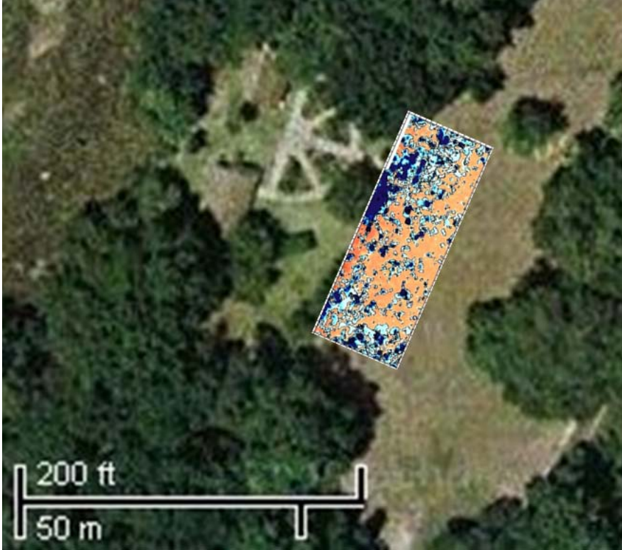
Figure 10. GPR Overlay Map (37-40 ns) on Aerial Image of Gascoigne Bluff Study Area.
