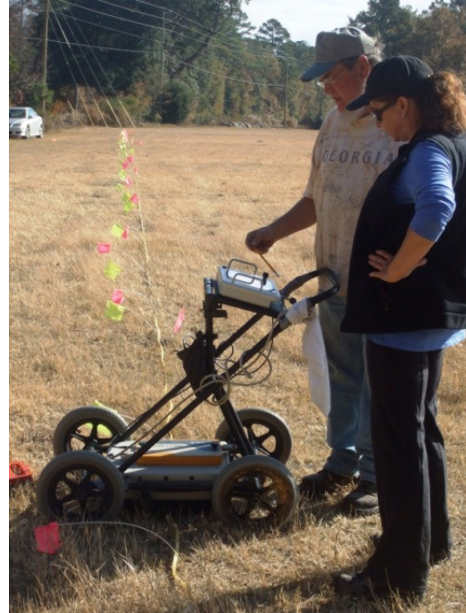
Figure 18. View of GPR Data Collection in Progress, Block A, Monteith Swamp.
