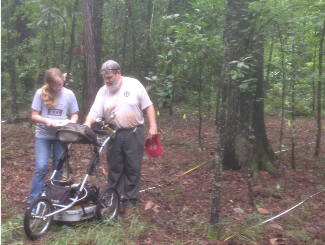
Figure 2. GPR Survey in Progress on Boyd Property.
