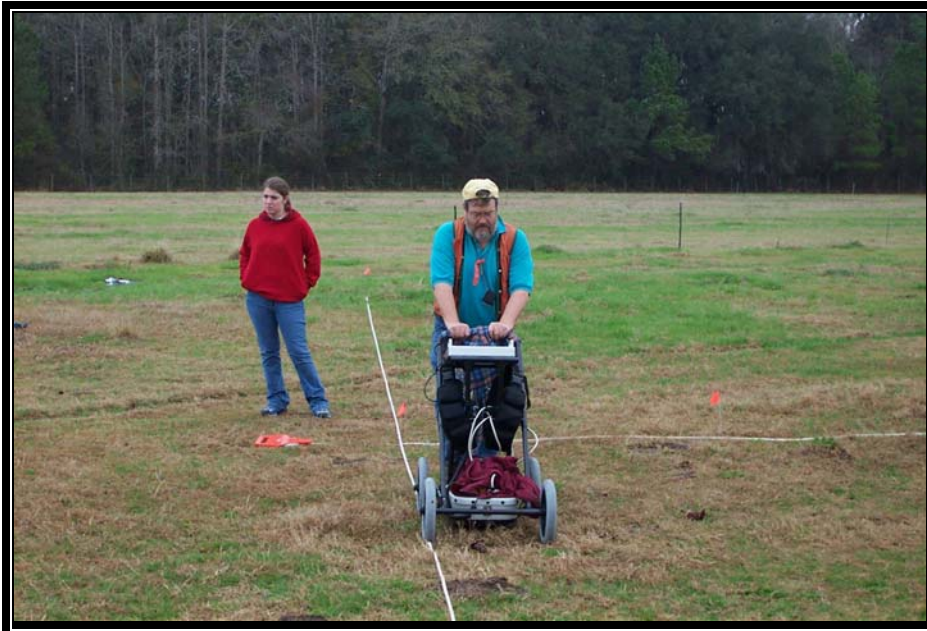
Figure 4. GPR Survey in Progress.
