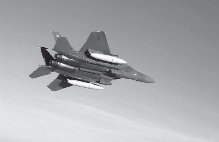
External fuel tanks on an F-15, a key enhancement demand of Saudi Arabia for the fighters it planned to purchase from the United States. (RG 330, NARA II)
