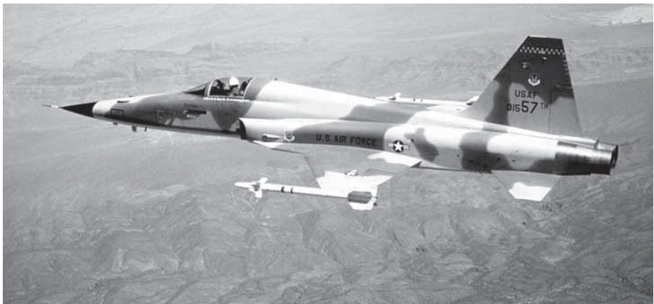
An F-5E Tiger II fighter carrying AIM-9 Sidewinder missiles, November 1981. (RG 330, NARA II)
