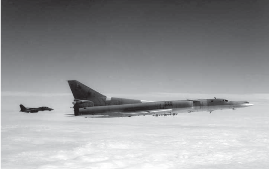
Soviet Backfire (Tupolev Tu-22M) bomber escorted by a U.S. F-14A Tomcat. (RG 330, NARA II)
