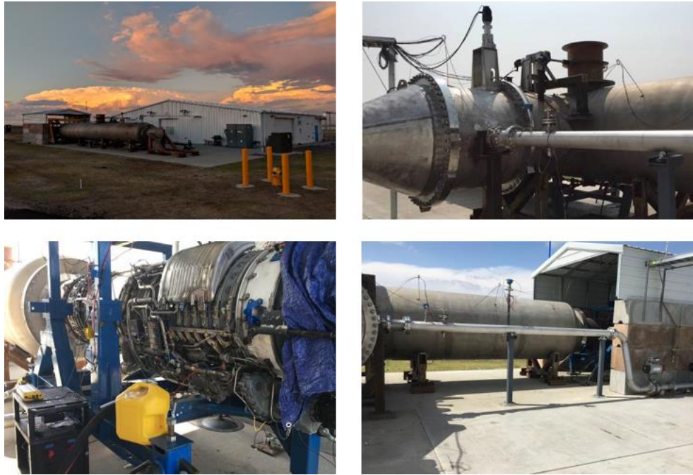
Figure 8: A selection of TF2 photos showing main plenum, assembly/test building and J79 jet engine.
