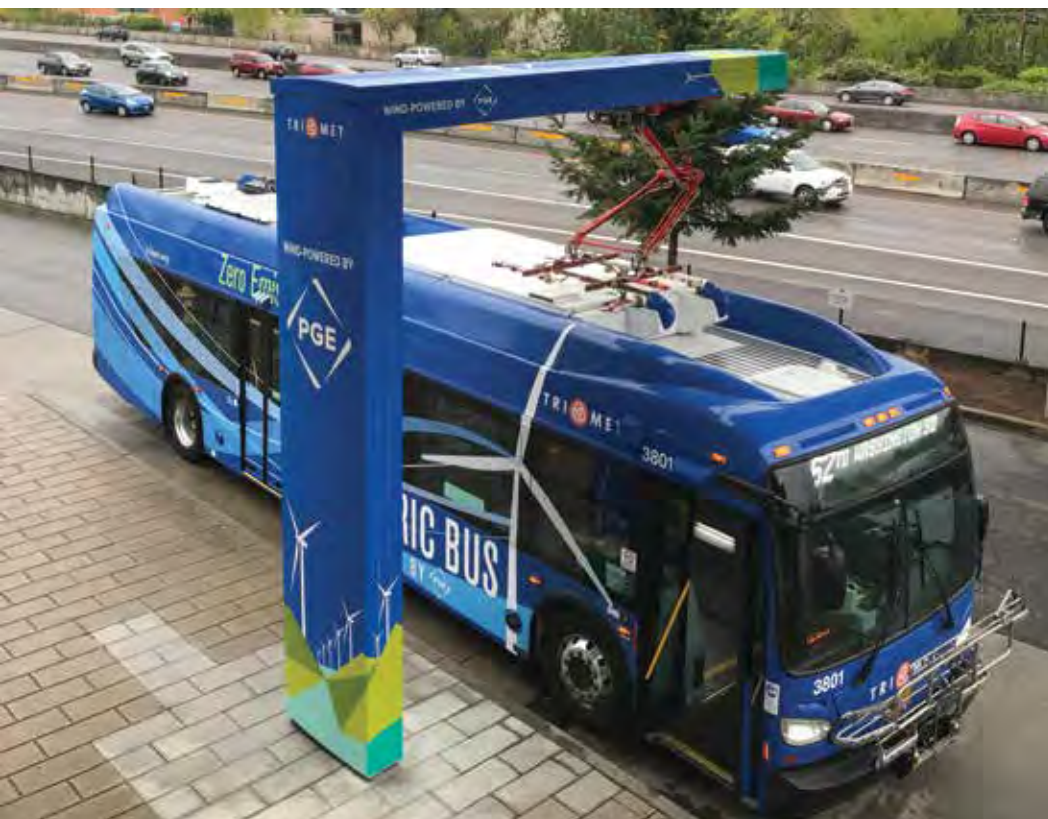
TriMet's first battery-electric bus charging at Sunset Transit Center (above) and on Line 62 (below)
