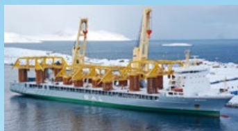
Unobstructed working deck of 128.50 × 27.50 m
