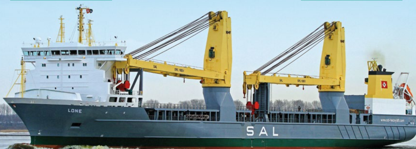
2 cranes of 1 000 t SWL lifting capacity each, in combination 2 000 t
