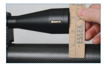
With the high mounted optics of an AR-type rifle, the close range impact will not follow the line of sight. A lot of new shooters are surprised by the results when they try to shoot at close targets. The gun will impact low at close range; enough to make a difference if you have a critical target. It can cost you points in a match, problems in a self-defense situation or, as happened to me, cause you to shoot under a bobcat that came in too close to the dying rabbit call.
