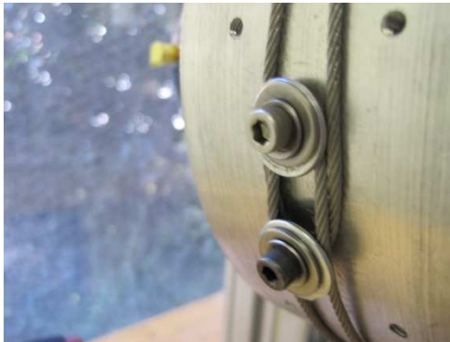
Figure 15: Drive rope termination point on drive sheave
