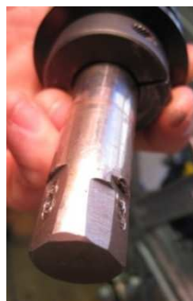
Figure 41: Flanges filed into shaft for bearing set screws
