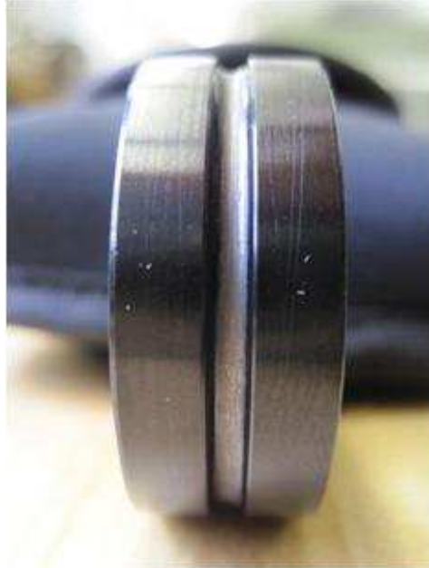
Figure 20: Groove wear pattern in anodized 6061-T6511 (No Teflon® Dip), by S.S. rope sample (16,300CTF)
