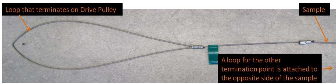
Figure 16: Drive ropes for wire rope samples
