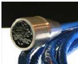
Figure 35: Potted fiber rope termination
