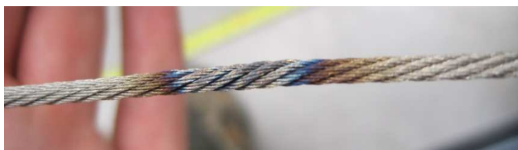
Figure 30: Torched 3/32" 7x49 stainless steel rope
