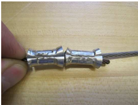
Figure 32: Crimped 1/8" sleeves over 2.5mm 7x49 tungsten rope
