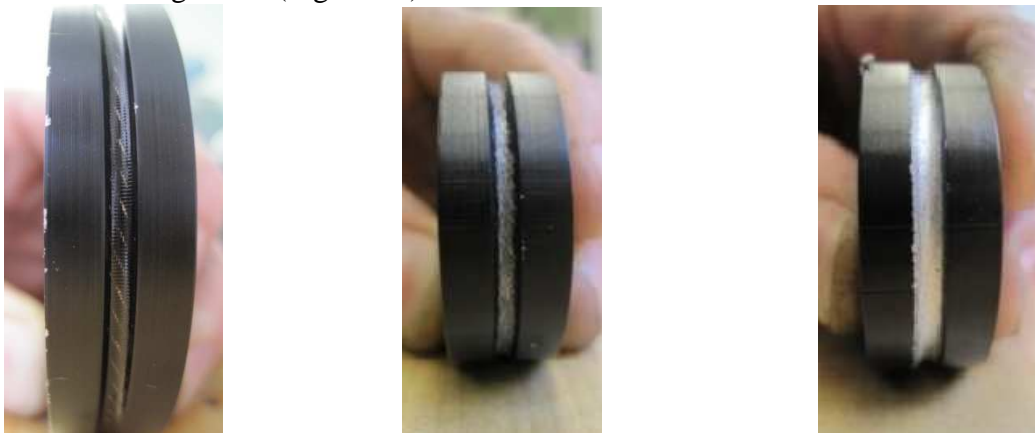
Figure 29: (Left to right) Chatter marked groove with wear pattern from 7x19 SS rope, tear out initiation of the groove, fully removed anodize coating.
