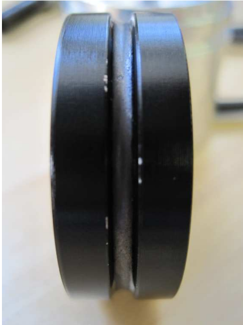
Figure 19: Wear induced by tungsten rope sample on an anodized 7061-T651 sheave (60,000CTF)
