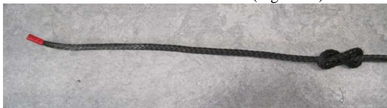
Figure 38: Initial Figure Eight knot setup
