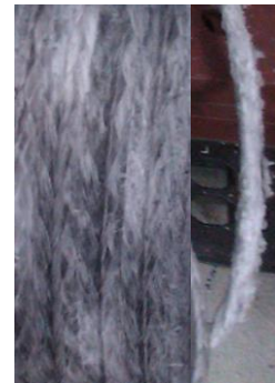
Figure 15: Abrasive damage at base layer (left) and upper layer (right).
