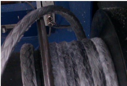
Figure 14: Deformation of base layer rope.
