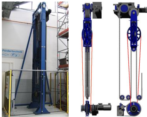
Figure 9: Test machine for winding tests.
