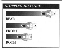
lever firmly and progressively. If the front wheel locks, release the front brake immediately, then reapply it firmly. At the same time, press down on the rear brake. If you accidentally lock the rear brake on a good traction surface, keep it locked until you have completely stopped. Even with a locked rear wheel, you can control the motorcycle on a straightaway *if it is upright and going in a straight line*.
