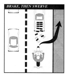
the side of your intended direction of escape. This will cause the motorcycle to lean quickly. Maintain pressure until the motorcycle has cleared the obstacle.
