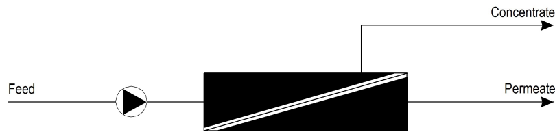
Figure 29. Continuous RO process
