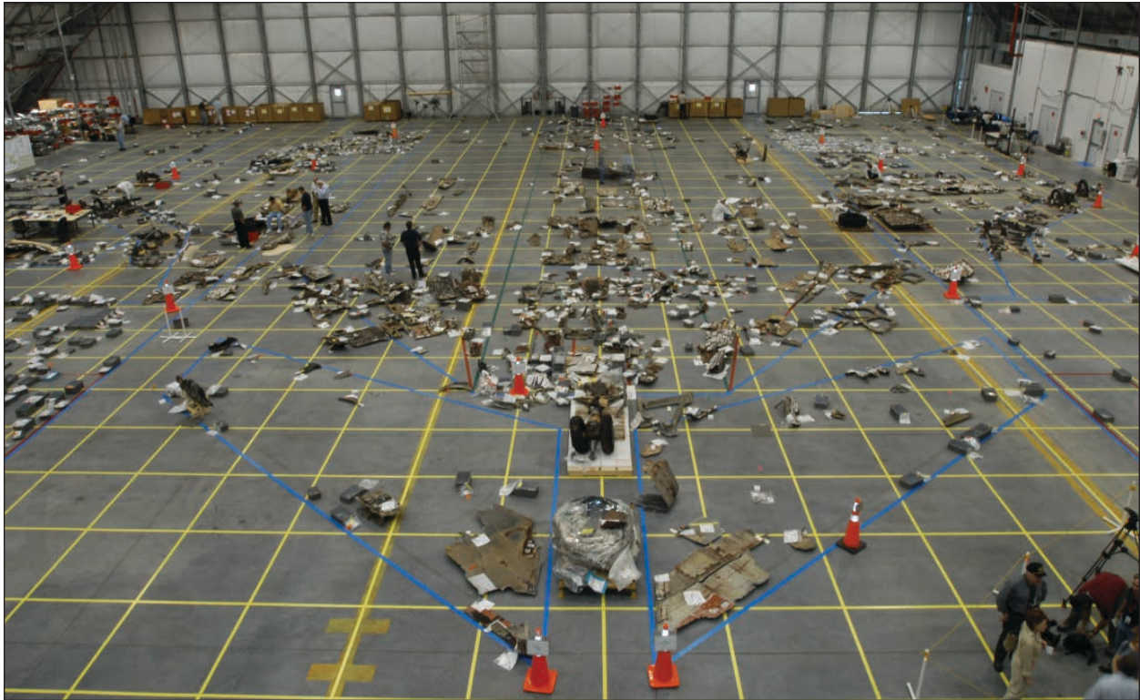
Reconstruction of the Columbia from parts found in East Texas and western Louisiana. From this layout, NASA was able to determine that a large hole occurred in the leading edge of the wing and identify the burn patterns that eventually led to the destruction of the orbiter.
