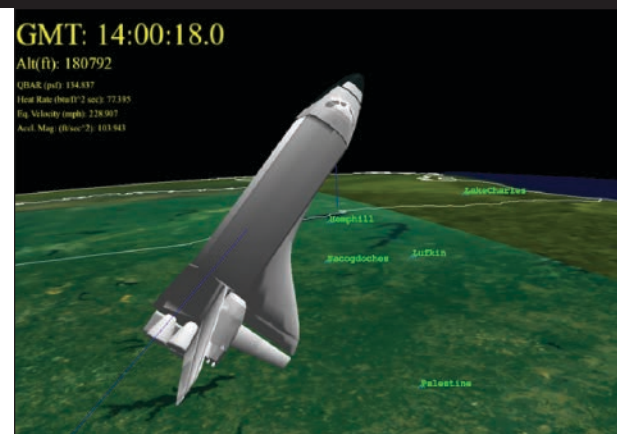
The Catastrophic Event (CE) was a period of time during which the orbiter vehicle was undergoing a major structural breakup. At this time, the accelerations on the forebody were estimated to be 3.5 Gs. The breakup sequence progressed over several seconds. Analysis of ground-based video of the event established the first detectable signs at GMT 14:00:18.
