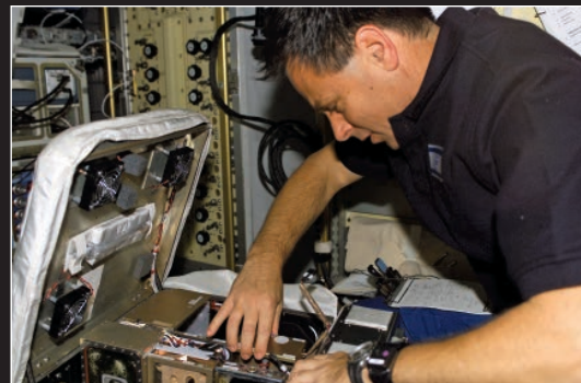
STS-107 Payload Specialist Ilan Ramon works with the Space Technology And Research Students (STARS) educational payload housed in an Isothermal Containment Module (ICM) in the SPACEHAB Research Double Module. The STARS payload included the following experiments: "The Chemical Garden," sponsored by Israel; "Astrospiders — Spiders in Space," sponsored by Australia; "Silkworm Lifecycle During Space Flight" sponsored by China; "Flight of the Medaka Fish," sponsored by Japan; "Carpenter Bees in Space," sponsored by Liechtenstein; and "Ant Colony," sponsored by the United States.
