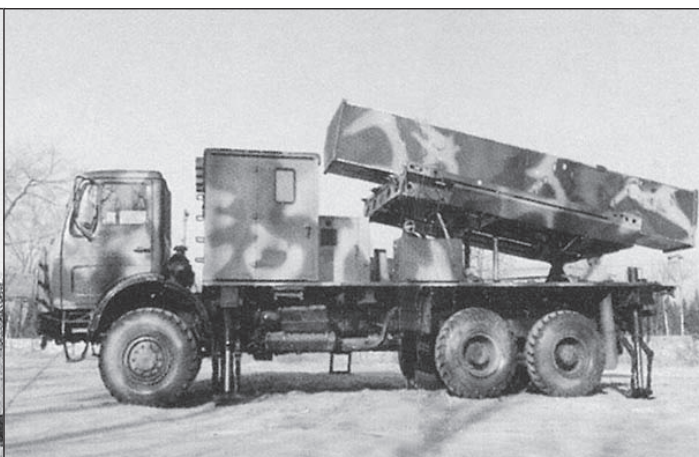
(From left to right) The radar/command truck needed to launch the C-802 (Noor) missile with the launcher vehicle (right). Missing is the third power generation truck needed to operate the missile in the land based configuration.
