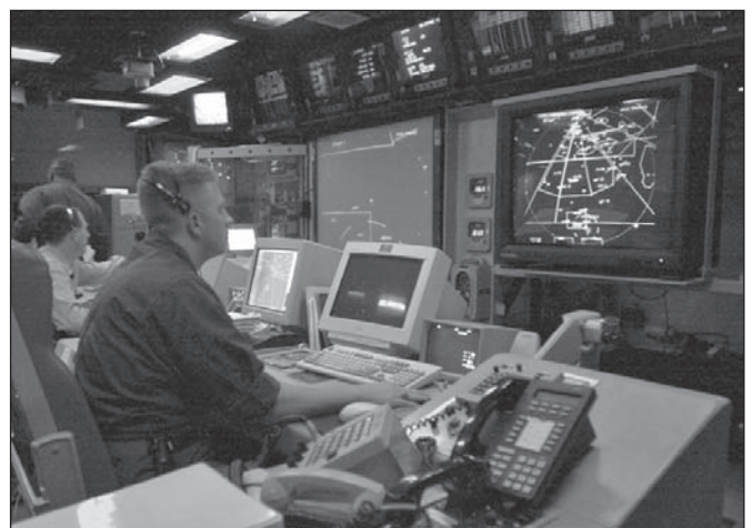
The operations room of a modern air warfare destroyer. Operations rooms such as these provide more workstation terminals, big screen theatre wide displays and space for planning and execution of complex joint operations than found on an AEW&C aircraft. The destroyer can also loiter for months and provide its own protection. (USN)
