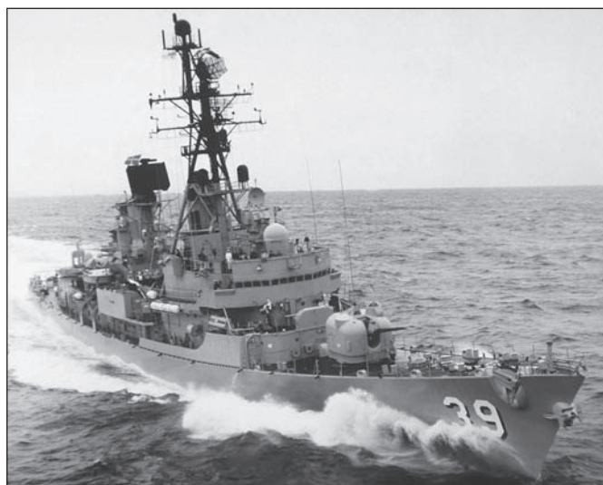
The Charles F. Adams class destroyer HMAS HOBART. The Adams class were originally designed to operate with Australia's aircraft carrier as a backstop to 'leakers'. However, when the carrier was decommissioned they became the principle means of air defence at sea. Something they were never really designed for given the limited anti-air missile magazine. (RAN)
