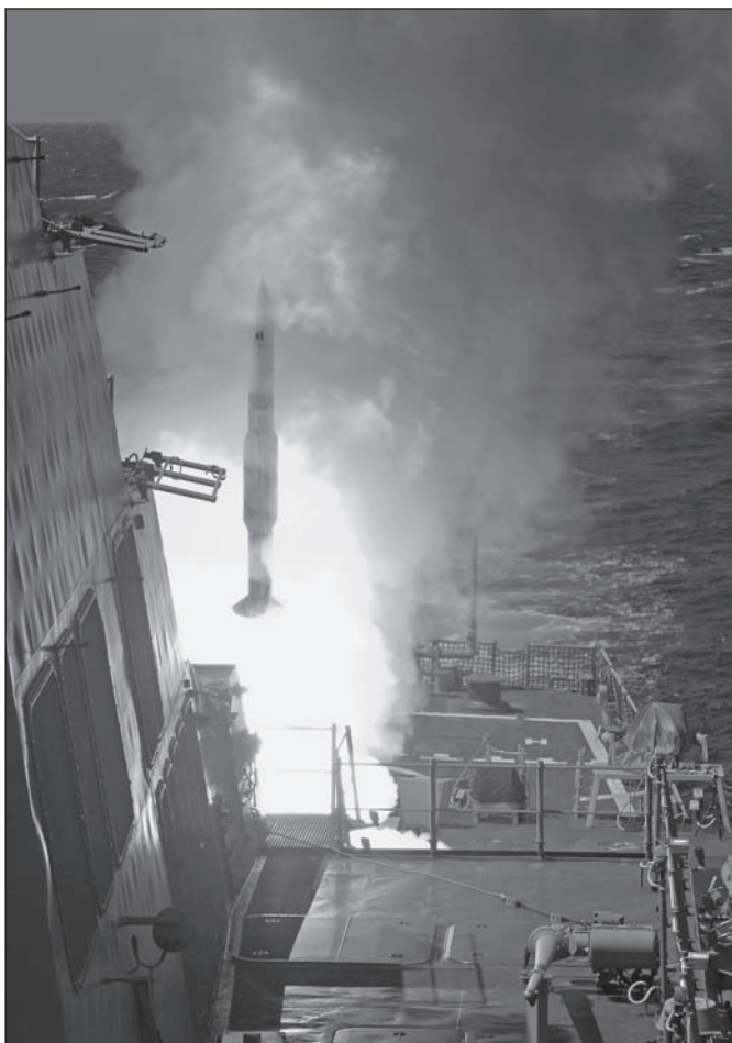
An SM-2 anti-air missile being fired from the USN Arleigh Burke class destroyer USS O'KANE during the recent RIMPAC 2006 exercise off Hawaii. The SM-2 has considerable advantages over the current SM-1 used by the RAN. Apart from being far more accurate and reliable its range is more than doubled, and it can permit the firing ship to handle a considerable number of targets simultaneously through its autopilot enabling time-sharing of the illuminator. (USN)
