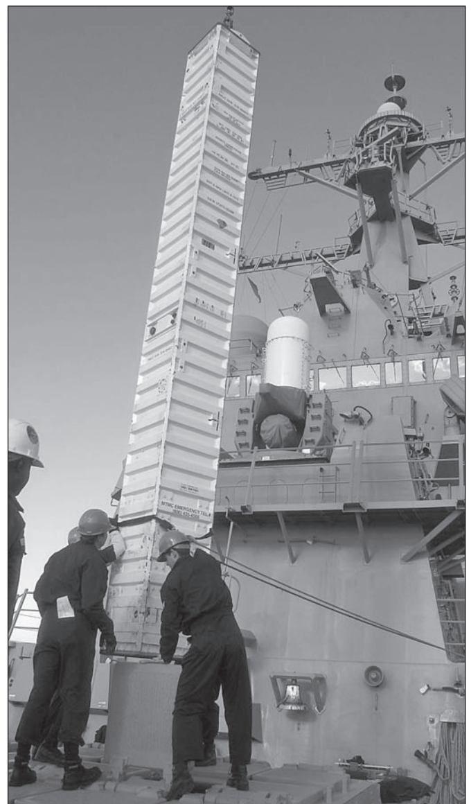
Crew members loading an SM-2 missile into its cell position in the forward Mk-41 VLS of an Arleigh Burke class destroyer. Given the awkwardness of the operation (i.e. weight and length of the launch canister) it is generally only done tied up to a dock. (USN)
