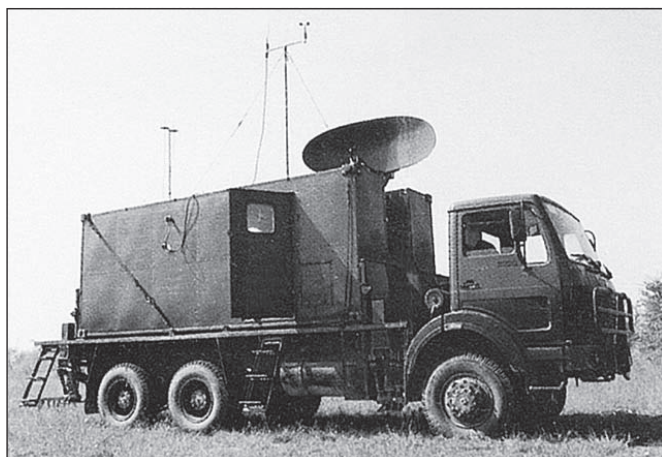
(From left to right) The radar/command truck needed to launch the C-802 (Noor) missile with the launcher vehicle (right). Missing is the third power generation truck needed to operate the missile in the land based configuration.
