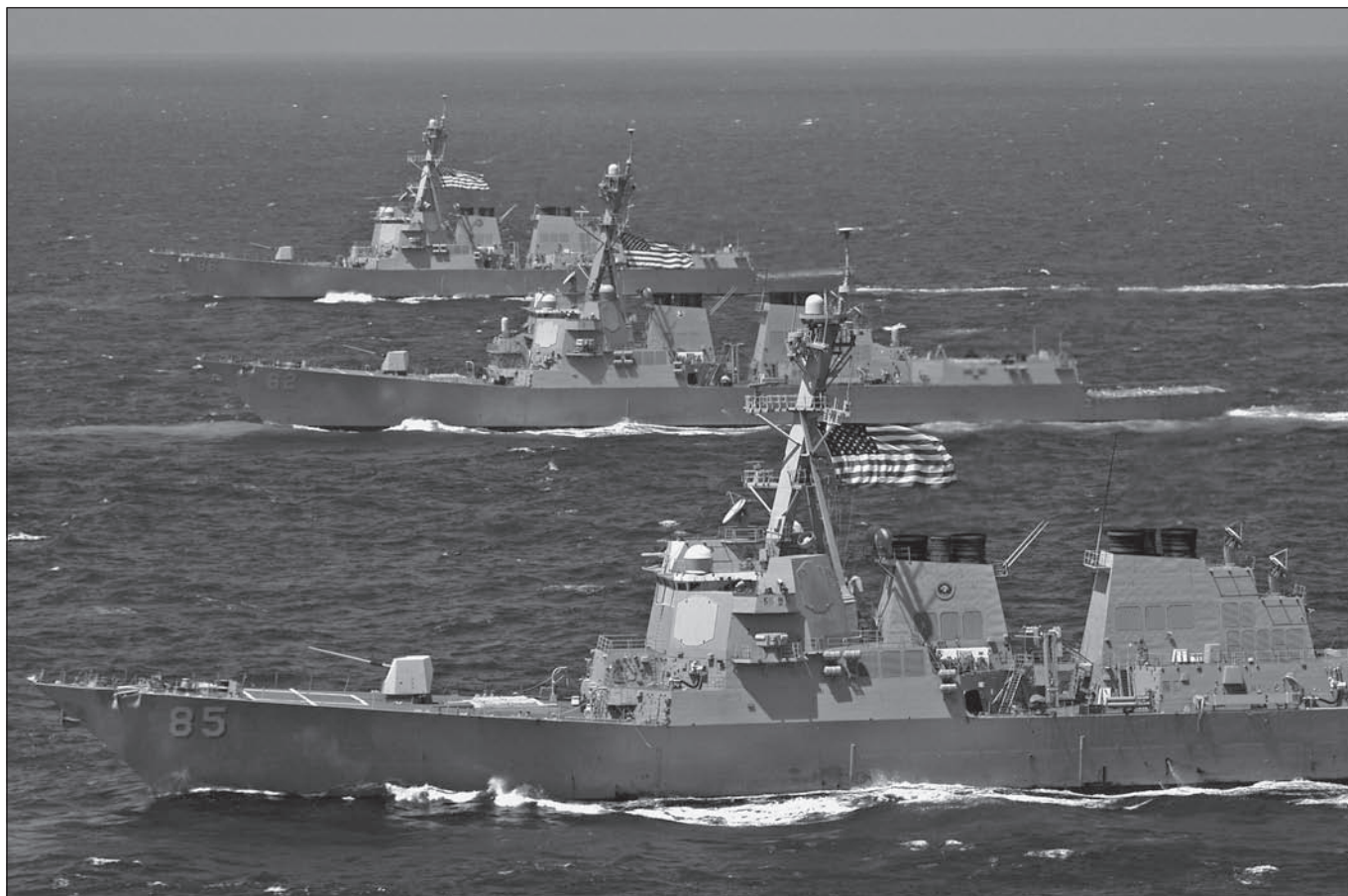
Three USN Flight IIA Arleigh Burke class destroyers at sea. The Arleigh Burke's each have nearly 100 vertical launch cells for many different weapons such as SM-2 and Tomahawk. This makes them more flexible for operations around the world. (USN)
