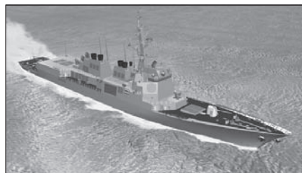
A computer generated image of the South Korean Navy's KDX-III destroyer. The KDX-III is a larger and more capable USN Flight IIA Arleigh Burke class destroyer. However, the KDX-III could more accurately be called a cruiser.
