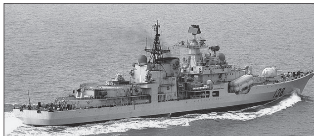
China's fourth Sovremenny class destroyer from Russia transiting the Indian Ocean. Note the absence of the aft twin 130mm gun mount and the two Kashtan CIWS either side of the entrance to the helicopter hanger replacing the numerous AK-630 Gatling guns.
