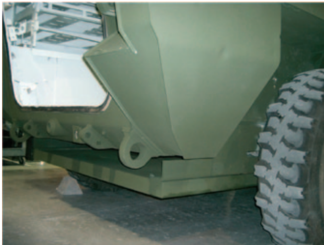
Expedient Stryker underside armor.
