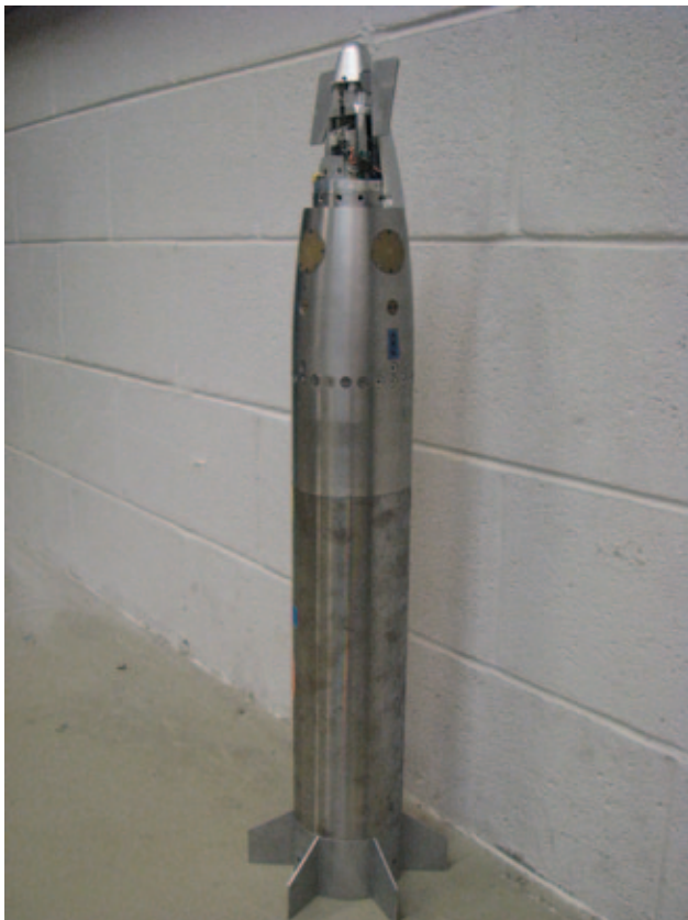
VAPP model: A launch and flight test bed was developed to support demonstration of VAPP technologies. The 105mm, fin-stabilized projectile shown is composed of a canard control mechanism, gun-hardened miniaturized electronics and embedded flight control algorithms. All components were developed and built at the Army Research Laboratory.
