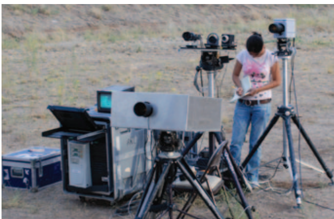
Erika Jackson, an ARL engineer, operates signature measurement equipment during field testing, which was used to measure mortar, small arms, and RPG signatures.
