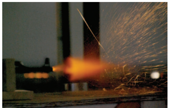
Long-time integration image of small arms muzzle flash taken during ARL signature measurements, which were used for emission characterization.
