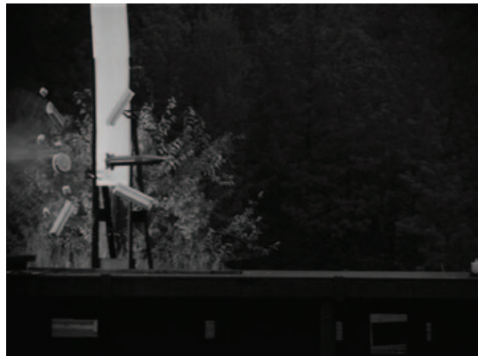
VAPP flight test: Free-flight experiments conducted at the Transonic Experimental Facility were the first to successfully maneuver a government-designed artillery projectile.
