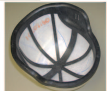
Graphite/epoxy stiffener applied to a polyethylene/aramid helmet.
