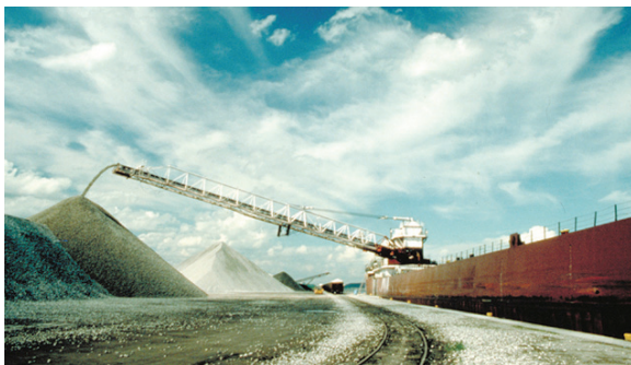
A modern bulk freighter self-unloads bulk cargo
