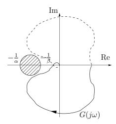
Figure 5: Circle criterion for open-loop stable system.
