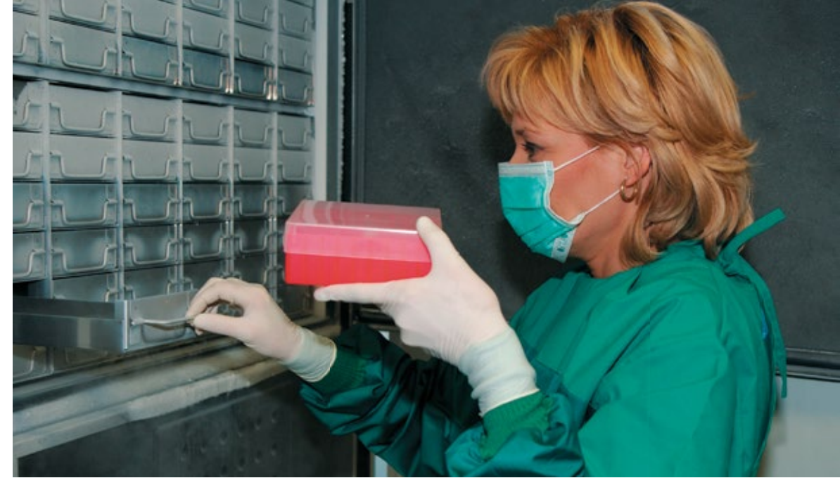
Many biological materials can only be stored at very low temperatures. Arranged neatly, everything can be found easily, even at –80 degrees Celsius
