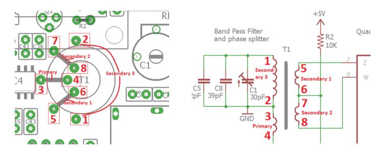
On the following page is a diagram hand-drawn by Ed WA4MZS (thanks Ed!) which may also clarify the construction and installation of T1.
