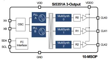
Voltage Controlled Oscillator in the range 600-900MHz (the PLL), then divided down to produce the final output frequency. The multiplication up and the division own are both fractional and so the frequency resolution is extremely finely controlled. The chip has two PLLs and three output divider units.
