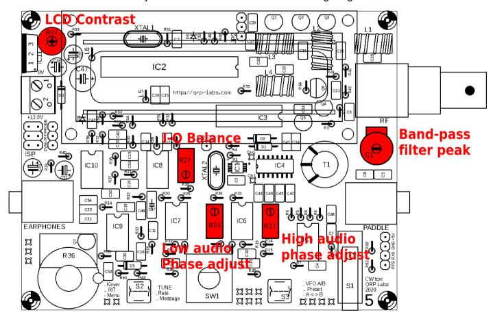
In summary: the alignment tools built into the radio consist of a signal generator which injects a signal into the RF front end, and digital signal processing which adds a 250-Hz digital filter to the
