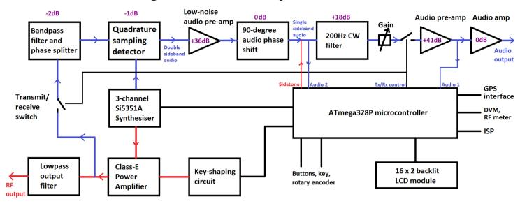
This CW transceiver is a high performance, yet simple and low cost, analogue design. The transmitter uses a high efficiency Class-E amplifier which results in low current draw on transmit, and inexpensive transistors with no heatsinks.
