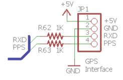
The optional GPS interface is provided by a 4-pin header at the bottom right of the board, next to the 3.5mm socket for the keyer. The pinout of the 4-pin header exactly matches the one on the QRP Labs Ultimate3S QRSS/WSPR transmitter kit, and the QRP Labs QLG1 GPS receiver kit. This makes connecting the radio to the QLG1 GPS kit very easy, if you wish. However other GPS modules could also be used. The following requirements of the
