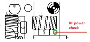
At the top right corner of the PCB, you will find a pad on the PCB where the L1 wire is soldered in. This pad is connected directly to the RF output pin of the BNC connector (see diagram). If you connect a wire from here, to pin 2 of the 3-pin DVM/RF Power header, then key-down, the display will read the power output in Watts. It is easiest to have the transceiver in Straight key mode and just press the microswitch.
