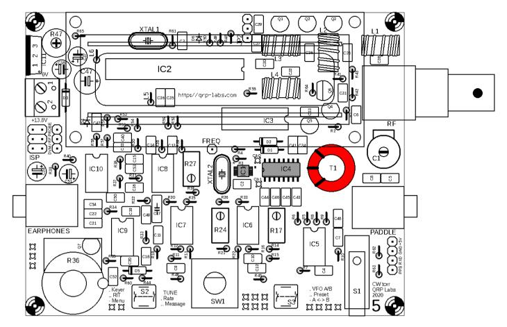
The number of turns in each winding depends on the band you are building the kit for. Refer to the following table. For convenience, the remainder of the instructions in this section refer to the 20m version (30 + 3 + 3 + 3 turns).
