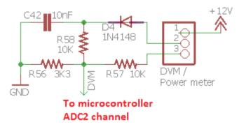
applies a division by a factor of 4.03. Since the ADC can measure voltages up to 5V, this means the DVM function has a range of 0V to 20V maximum, and each ADC bit has a resolution of 0.02V.
