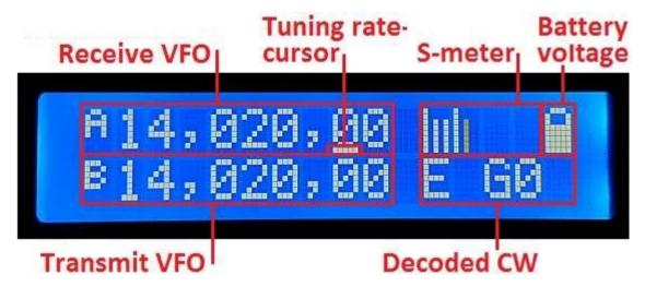
The main display layout during ordinary operation (which will be called "main operating mode") is shown in the above photograph. The display during beacon or message transmission modes, menu editing, alignment etc. differs. The main display elements are as follows:
