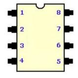
Where an IC pin number is mentioned, remember that pin numbers start from the top left (just to the left of the dimple at the end of the chip) and are counted anticlockwise from there (see diagram of 8-pin IC for example, right).
