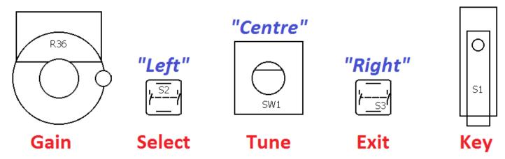
This diagram shows the operating controls of the radio. All of the controls except the Gain potentiometer have multiple functions, depending on the operating mode, menu editing, etc. The tuning rotary encoder in the centre has a button on its shaft that is activated by pressing it, and this button also has multiple functions.
