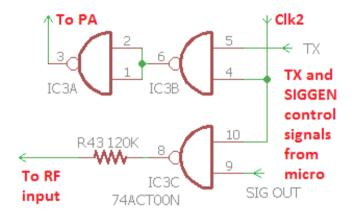
configuration. However, this transceiver design also includes the built-in signal generator feature, for aligning the Band Pass Filter and adjusting the I-Q balance and phase adjustment controls. So, some of the spare gates in the 74ACT00 are used to switch the signal generator on/off and the RF Power Amplifier (PA) signal on/off, separately.
