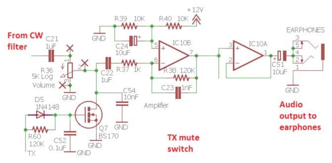
There is also a TX mute switch formed by Q7, another BS170 MOSFET. This was a late addition to the design: despite all attempts, I could not remove the nasty click on receive/transmit switching. The mute switch helps to attenuate it. The switch is operated by the microcontroller Receive/Transmit switch output. When the BS170 switch is on, it has a low resistance to ground which greatly attenuates the audio signal.
