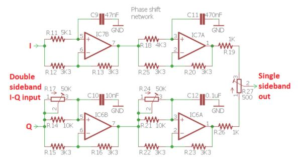
By this stage the I and Q outputs are each double-sideband, and we need to process them to demodulate single sideband.
