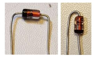
case of D1, D2 and D5, the PCB silkscreen printing shows a white stripe at the end of the diode body which must match the black stripe on the left end of the diode (photo above).
