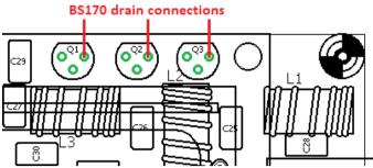
If you see power output at the BS170 drains, but not at the overall transceiver RF output, then this means that the fault lies in the Low Pass Filter. Check the soldering and the enamel situation, on those toroids.
