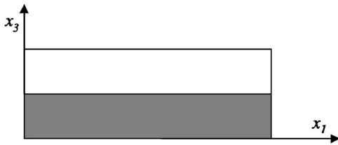
FIG. 6. A simple bilayer composite of piezoelectric and magnetostrictive layers.
