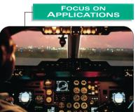
• **INSTRUMENT** PANEL In addition to gauges that give speed and altitude readings, the instrument panel of an airplane also contains an *attitude indicator*. This instrument tells how the airplane is tilted in relation to Earth's horizon.
