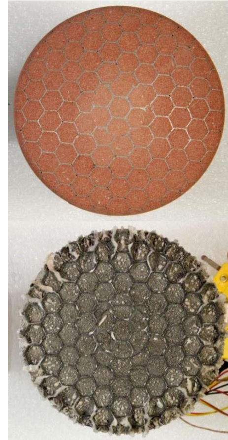
Before and after Avcoat arc jet models
