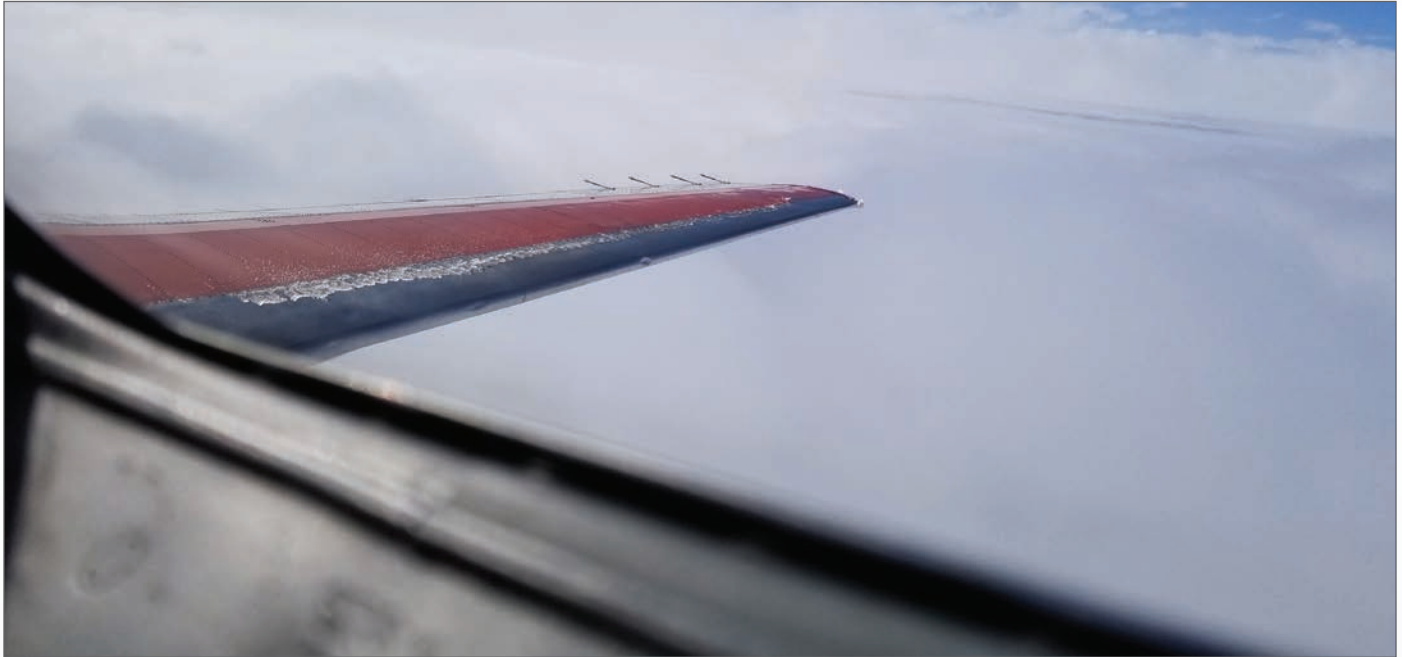
Runback icing on Convair wing during flight.
