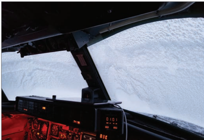
Convair windshield iced up in flight.
