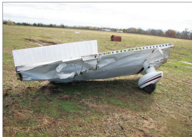
A section of the left wing from a Cherokee Six that suffered an inflight breakup due to a weather encounter.
