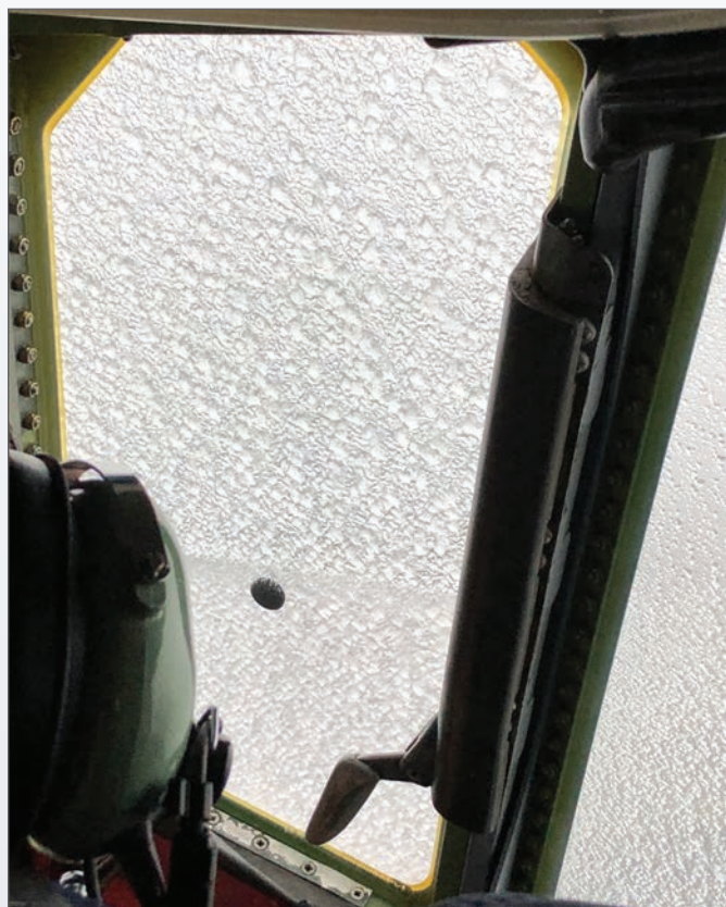
Convair side-window icing indicative of supercooled large droplet SLD environment.
